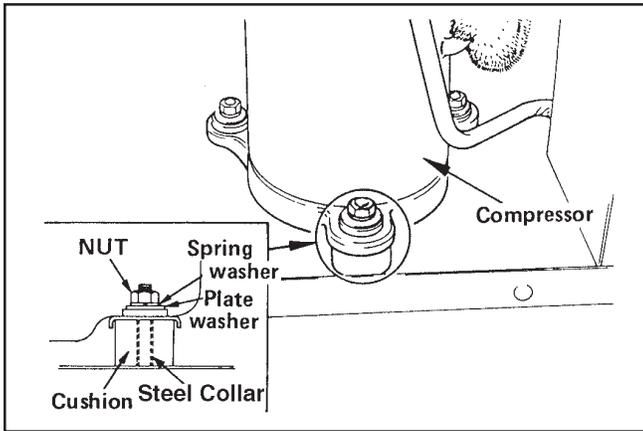
Reassemble the unit in the reverse order of removal. Described below are the parts that require special care in reassembling the unit. Perform all wiring or rewiring as referenced in the wiring diagram.
