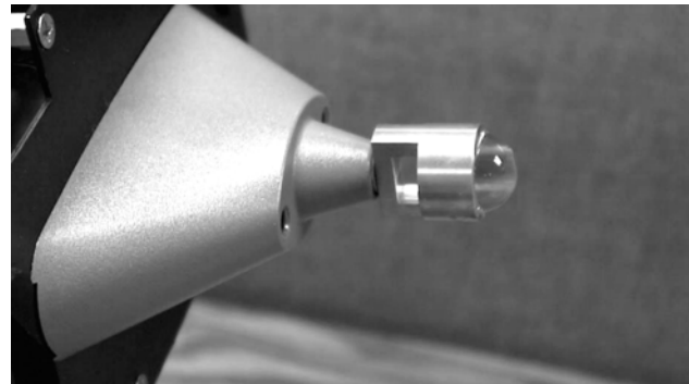
Figure CT-5. Glass Eye Fixture Installed
