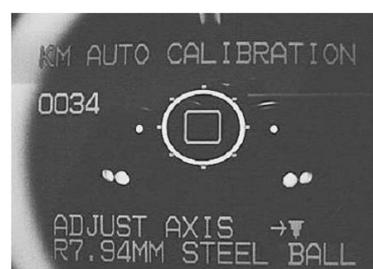
5. Perform the calibration with the steel balls of R5.95 mm, R7.94 mm and R9.13 mm.
