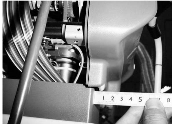
3. Hold the front cover by hand and measure the clearance between the front cover and M084 where there is no opening between the front plate (M302) and front cover.
