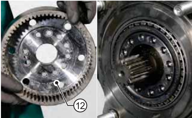
FIGURE 24: Match up the punch marks on the joint case and the crown wheel carrier flange.
