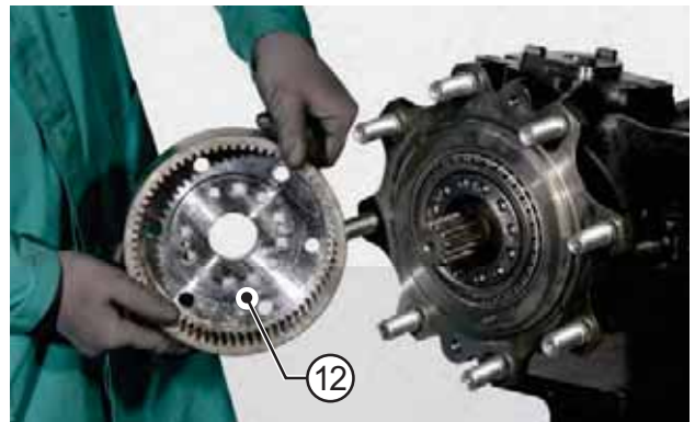
FIGURE 10: Remove the crown (13) with crown flange (12).
