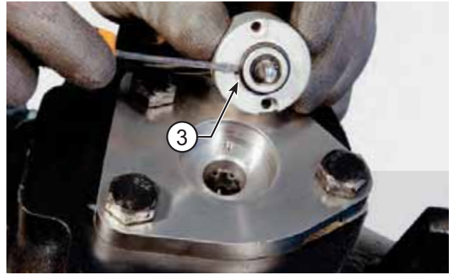
FIGURE 21: Place the sensor's o-ring (3).
