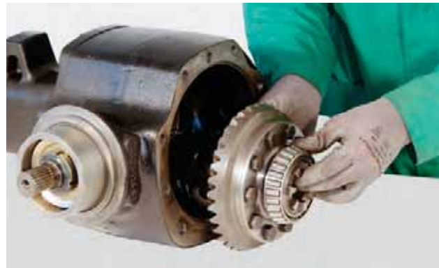
FIGURE 10: Extract the whole differential unit.
