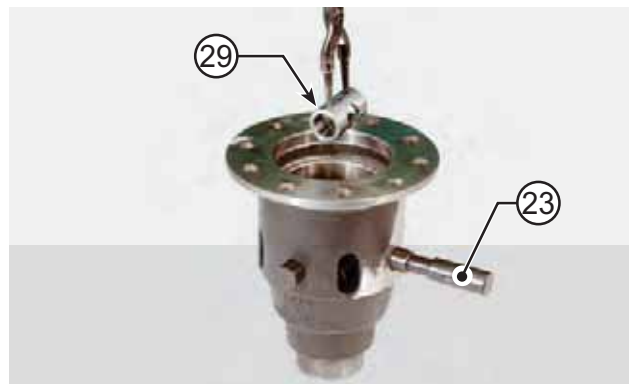
FIGURE 29: Insert the crossbolt (29) in the correct position.
