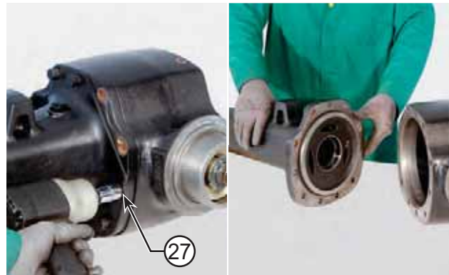
FIGURE 22: Connect a suitable lifting system. Loosen and remove the screws (27) securing the arm to the body. Remove the arm.
