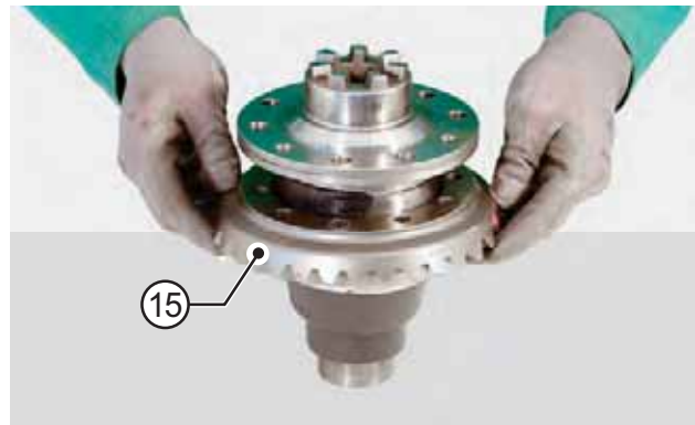
FIGURE 34: Position the crown (15) on the differential carrier and lock it with screws (14).
