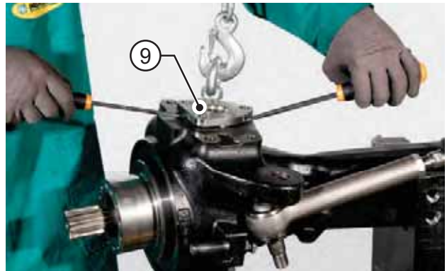
FIGURE 5: Remove the upper kingpin (2) complete with front seal (4) and shims (3).
