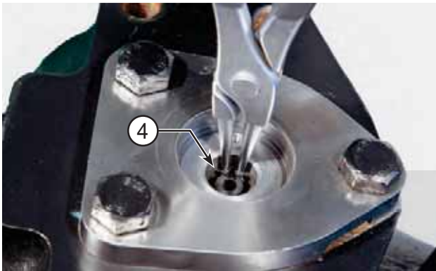
FIGURE 20: Install the snap ring (4).
