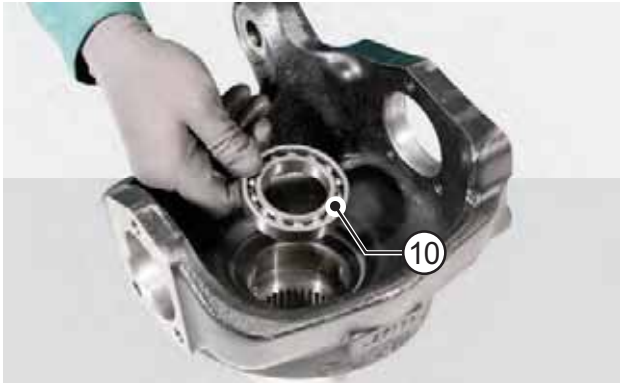
FIGURE 13: Using a puller, remove the bearing (10) from the steering knuckle.
