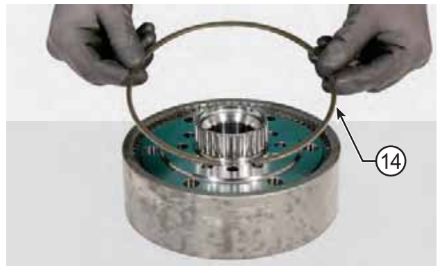
FIGURE 11: Remove the snap ring (14) from the crown (13).
