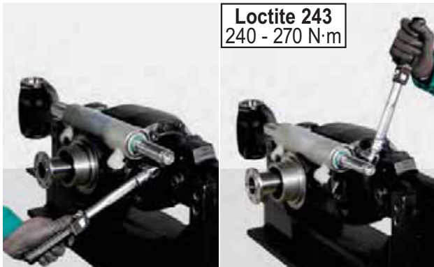
FIGURE 22: Lock the cylinder (5) screws (4) using the criss-cross method. Apply Loctite 243 to the thread. Torque wrench setting: 240 - 270 N·m
