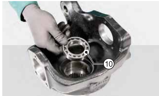
FIGURE 19: Insert the bearing (10) in the steering knuckle.
