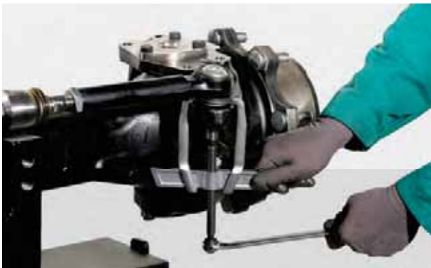
FIGURE 2: Disconnect the tapered pins of the tie rods (2) from the steering knuckle using a puller.
