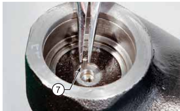
FIGURE 11: Remove the pin (7).
