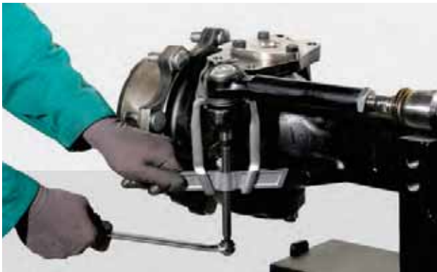
FIGURE 3: Disconnect the tapered pins of the tie rod from the steering knuckle using a puller.
