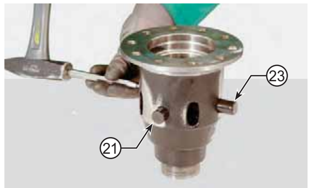
FIGURE 18: Remove the bolts (21) with the help of a drift.
