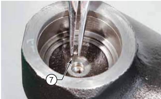
FIGURE 12: Insert the pin (7) in its seat.
