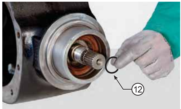
FIGURE 12: Use a screwdriver to remove the o-ring (12).
