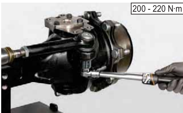
FIGURE 24: Insert the pins (2) in the steering case and lock into position using a torque wrench setting of 200 - 220 N·m.
