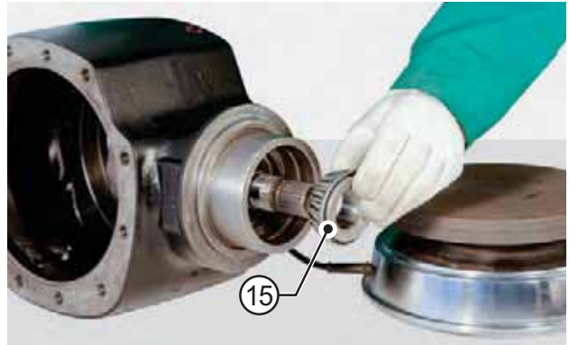
FIGURE 27: Heat the outer bearing (15) to a temperature of about 80C° and fit it on to the pinion (18).
