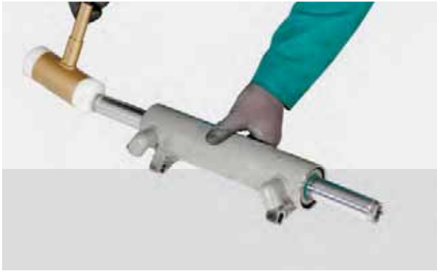
FIGURE 7: Hammer the piston on the rear of the head using a plastic hammer. Continue hammering until the head is ejected from the cylinder.
