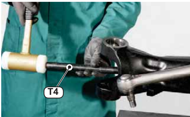
FIGURE 17: Lubricate and fit the sealing ring (14) onto tool T4 (See drawing T4 p. 69); install the rings into the arm.
