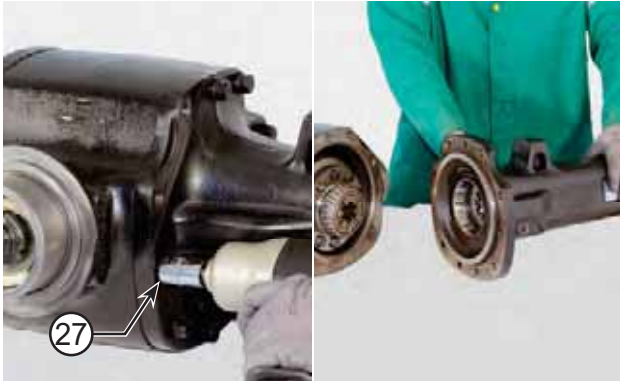
FIGURE 1: Connect a suitable lifting system. Loosen and remove the screws (27) securing the arm to the body. Remove the arm.
