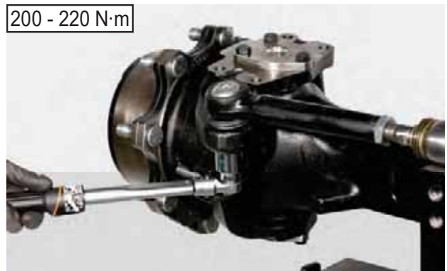
FIGURE 17: Insert the kingpins in the steering knuckle and lock into position using a torque wrench setting of 200 - 220 N·m.
