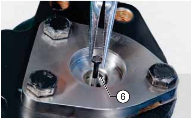
FIGURE 18: Lubricate and insert the sensor pin (6).
