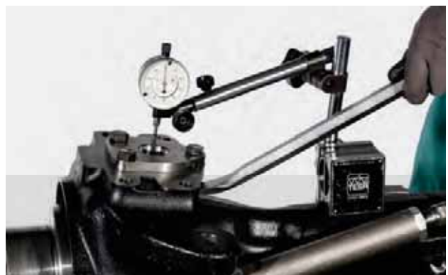
FIGURE 33: Check the vertical gap using a lever.
