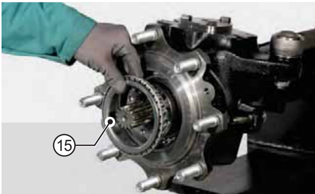
FIGURE 14: Remove the external bearing (15) and the hub (17).
