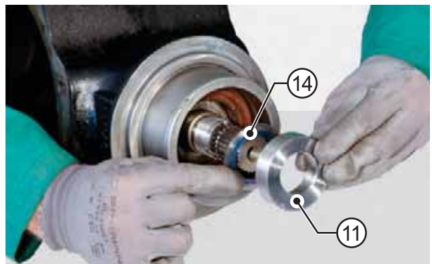
FIGURE 11: Remove spacer (11) and shims (14).
