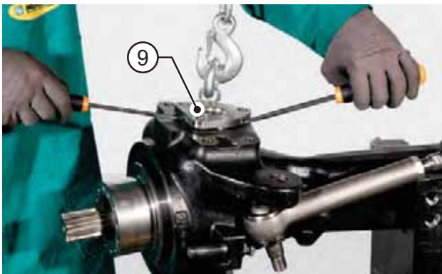
FIGURE 8: Remove the upper kingpin (9) complete with front seal ring and shims.
