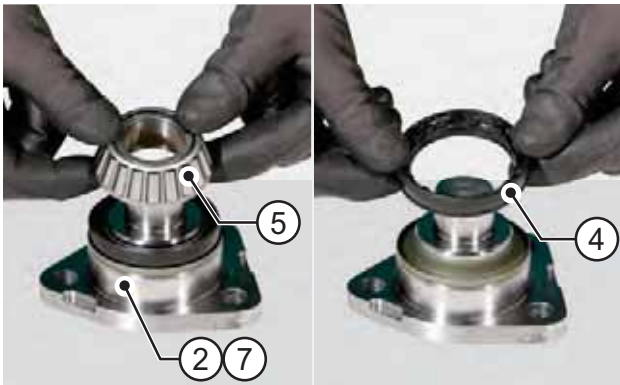
FIGURE 7: Remove the bearing (5) from the knuckle post (2, 7). Remove the sealing ring (4) from the knuckle post (2, 7).
