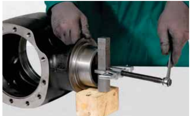
FIGURE 17: Using an internal extractor, remove the thrust blocks (15, 17).
