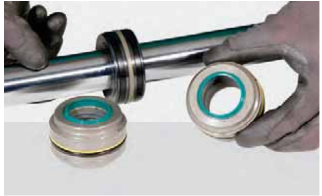
FIGURE 10: Remove all seals, anti-extrusion rings, and scraper rings from head, cylinder, and piston.
