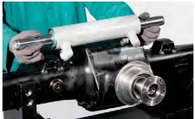
FIGURE 5: Extract the cylinder (5) using a plastic hammer.
