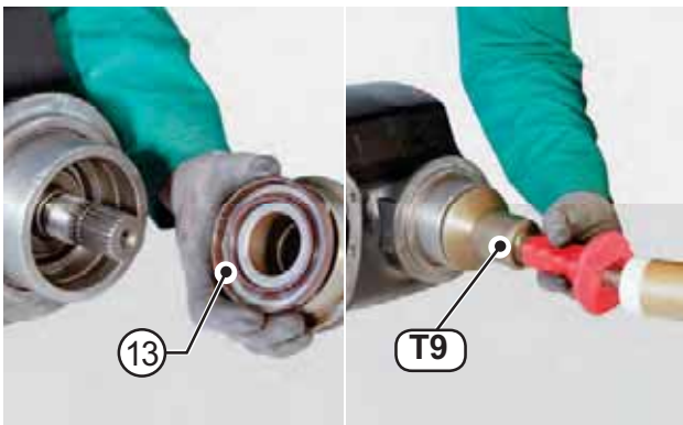
FIGURE 42: Lubricate and fit the sealing ring (13) onto tool T9 (See drawing T9 p. 73). Install the ring into the seat.
