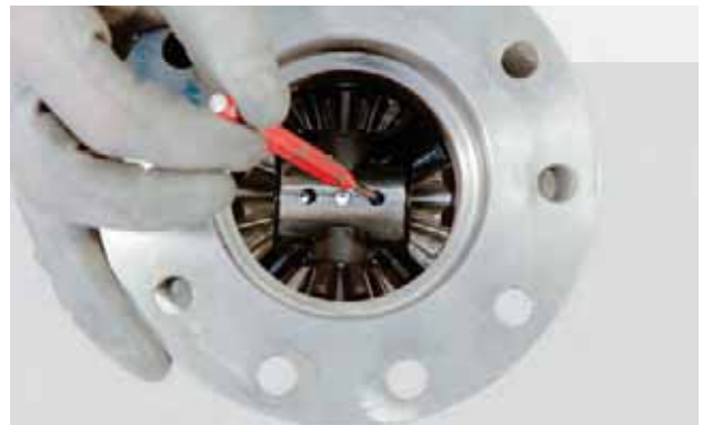
FIGURE 17: Move the two opposite mounted short bolts (21) to the outside of the box using the same pin driver.
