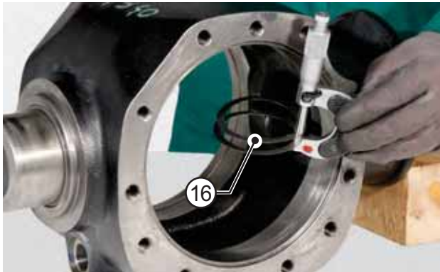
FIGURE 19: Check the thickness of first step pinion shims (16). Example: A = 1,1 \text{ mm}
