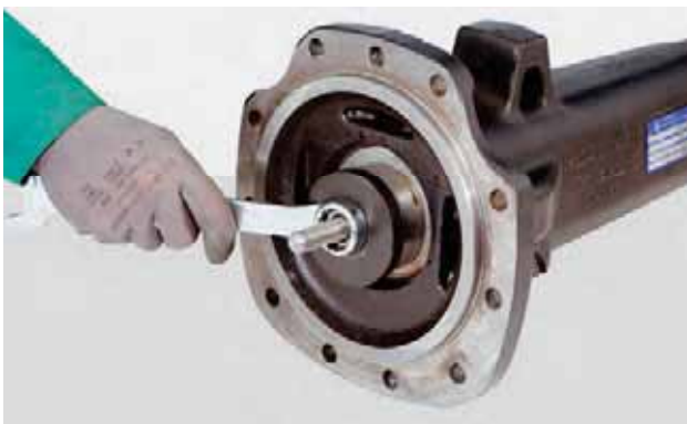
FIGURE 3: By acting on the buffer spring guide sleeve (10), tighten the nuts on the threaded rod, compressing the spring (8).
