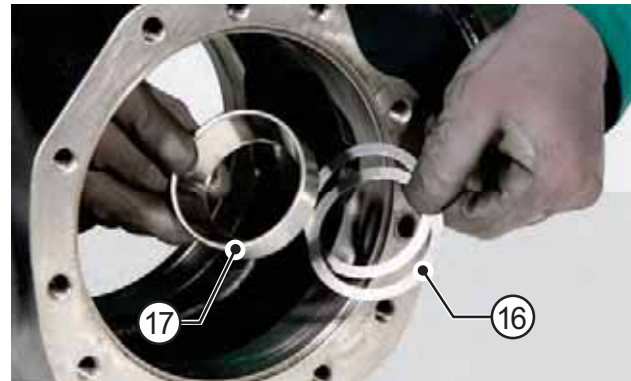
FIGURE 22: Partially insert the thrust block of the bearings (15, 17).
