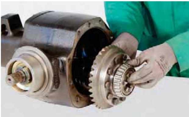
FIGURE 37: Install the whole differential unit.
