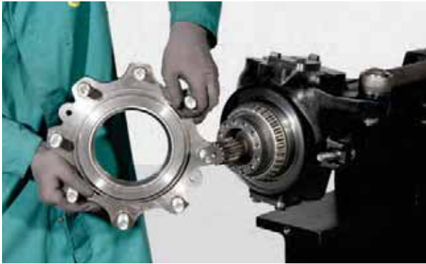
FIGURE 40: Fit the planetary gear cover onto the wheel hub. For details, see PLANETARY REDUCTION GEAR p. 15.
