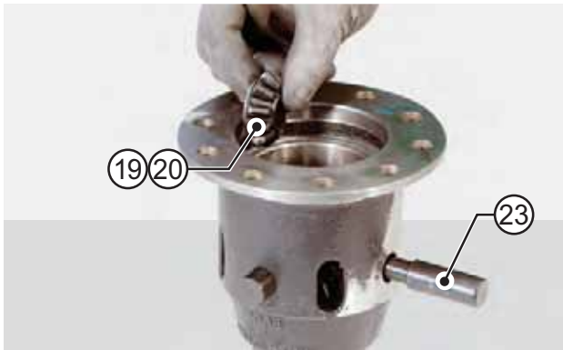
FIGURE 30: Satellite gears (20), spherical washers (19) and completely insert the long bolt (23).
