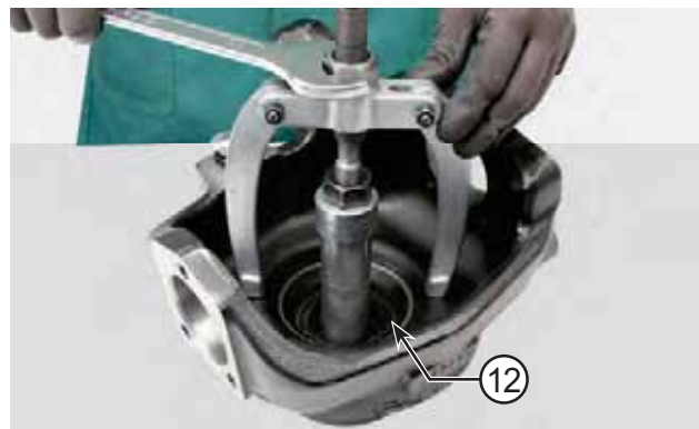
FIGURE 11: Using a puller, remove the sealing ring (12) from the steering knuckle.
