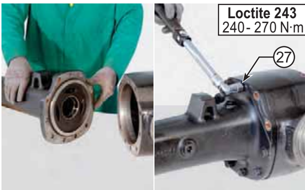
FIGURE 25: Insert a new o-ring on the centering diameter of the arm. Position the arm on the central body. Tighten nuts (27) in two stages, using the criss-cross method.
