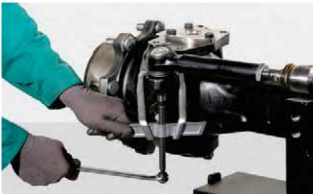
FIGURE 2: Disconnect the tapered pins of the tie rod from the steering knuckle using a puller.
