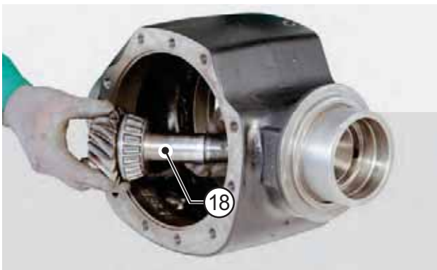
FIGURE 26: Fit the pinion (18) in the central body.
