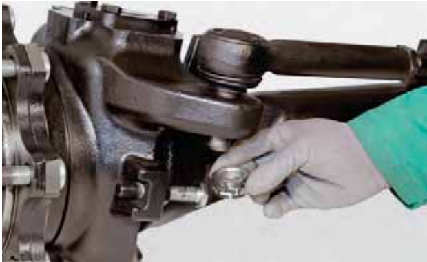
FIGURE 1: Remove the tie rod nuts.
