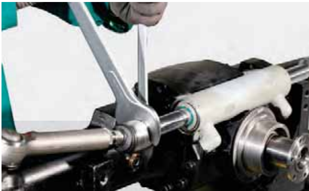
FIGURE 3: Disconnect steering bars (3) from the piston.
