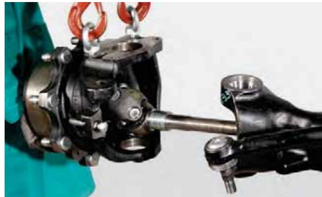
FIGURE 10: Remove the complete steering knuckle.
