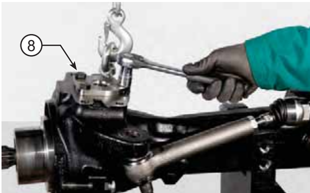
FIGURE 7: Loosen and remove the capscrews (8) from the kingpin (9).
