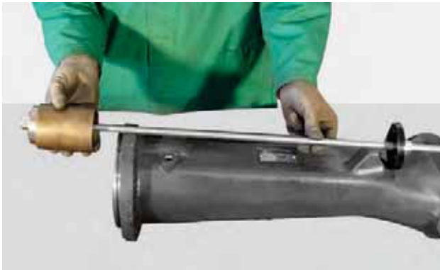
FIGURE 2: Insert an M14 threaded rod in the arm correlated with a swab from the appropriate diameter and a hard stop.
