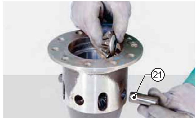
FIGURE 27: Insert the two half bolts (21), spherical washers (19) and satellite gears (20).
