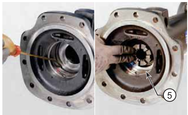
FIGURE 41: Lubricate the piston seating. Install the piston pack. Tap lightly with a mallet to seat the piston (5) completely. Mind the position of assembly.
