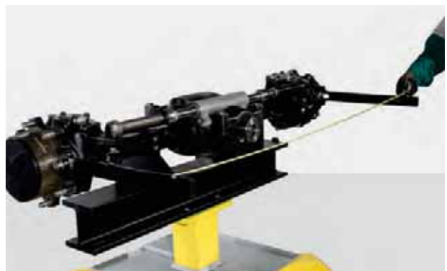
FIGURE 27: Without moving the piston, check front and rear distance at the edge of tools. Max. difference: = 2 mm
