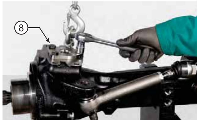
FIGURE 4: Loosen and remove the capscrews (1) from the kingpin (2).
