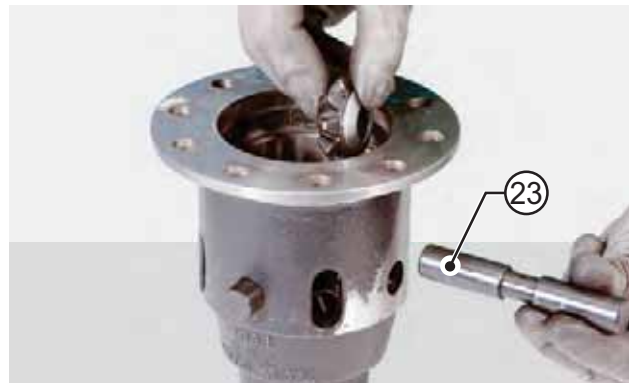
FIGURE 28: Partially insert the long bolt (23), satellite gears (20), and spherical washers (19).
