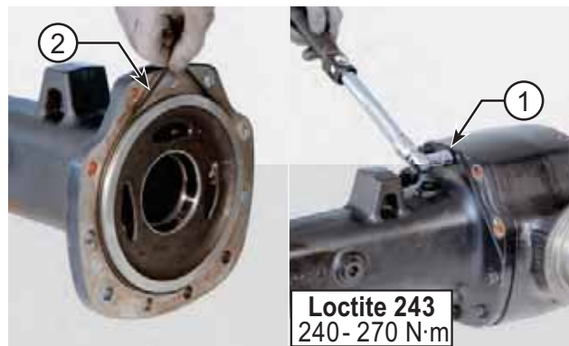
FIGURE 33: Insert a new o-ring (2) on the centering diameter of the arm. Position the arm on the central body. Tighten nuts (1) in two stages, using the criss-cross method.
