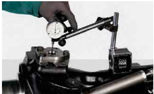
FIGURE 32: Position dial indicator, preset it to 1 mm and reset it to zero.
