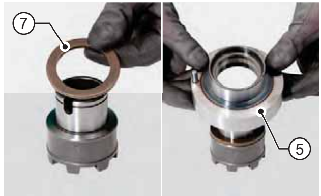
FIGURE 39: Fit in position the sleeve (9) complete with ring (7).
