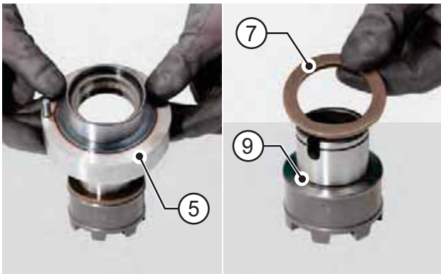
FIGURE 8: Remove the sleeve (9) and the relative ring (7).
