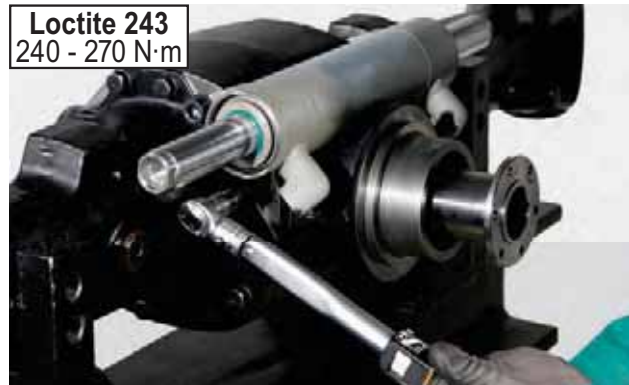
FIGURE 20: Lock the cylinder (5) screws (4) using the criss-cross method. Apply Loctite 243 to the thread. Torque wrench setting: 240 - 270 N·m
