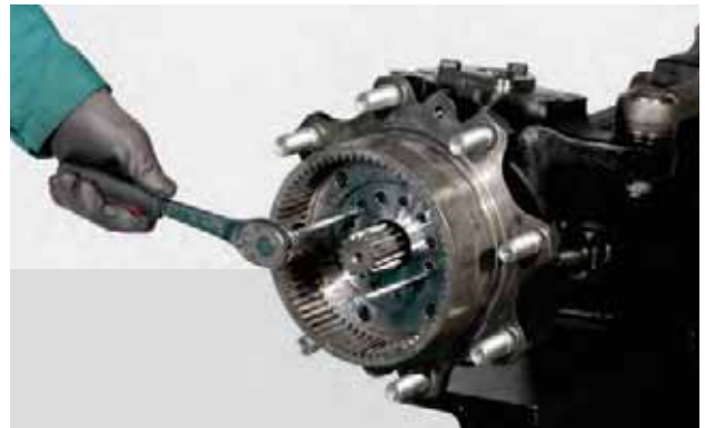
FIGURE 9: Tighten two M8 screws in the special threads. Tighten by one turn alternately.
