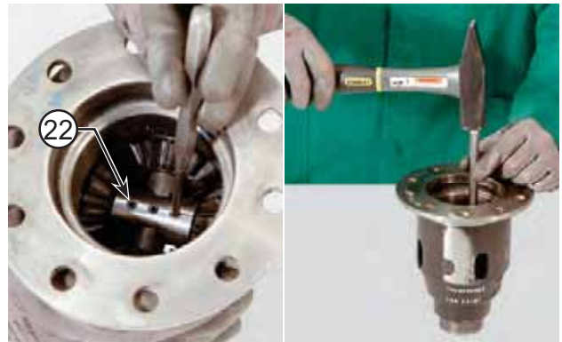
FIGURE 16: Remove the three spider blocking pins (22) by using a pin driver.
