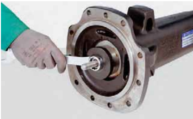
FIGURE 44: By acting on the buffer spring guide sleeve (10), tighten the nuts on the threaded rod, compressing the spring (8).
