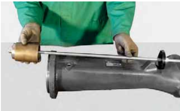
FIGURE 43: Insert an M14 threaded rod in the arm correlated with a swab from the appropriate diameter and a hard stop.
