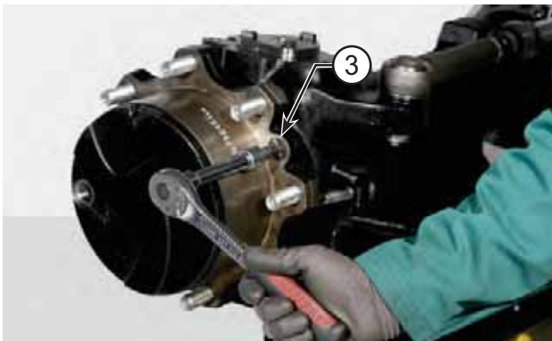
FIGURE 2: Remove the locking screws (3) of planetary cover (4).
