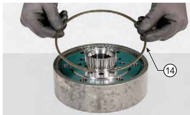
FIGURE 23: Insert the snap ring (14) in order to fix the flange (12) in the crown (13).
