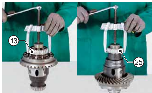
FIGURE 11: Extract the bearings (13, 25) from the differential carrier.
