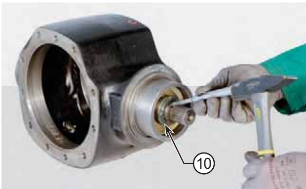
FIGURE 8: Remove the calking in order to preserve the screw cutting of the pinion during the ring nut (10) removal.
