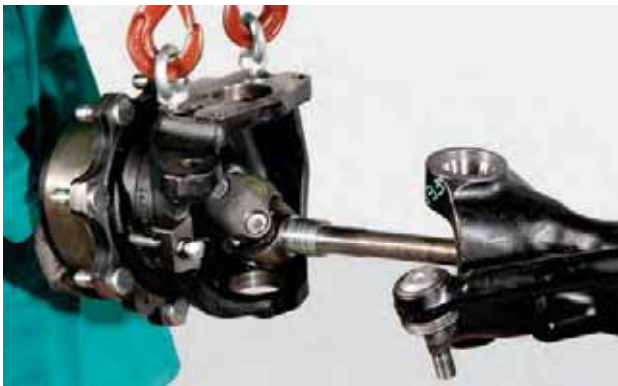
FIGURE 24: Tighten fully into the hole provided two double joint lifting eyes size M16, connect to suitable lifting gear and tighten. Pay attention not to damage the dust cover rings and the sealing rings. Install the steering knuckle.
