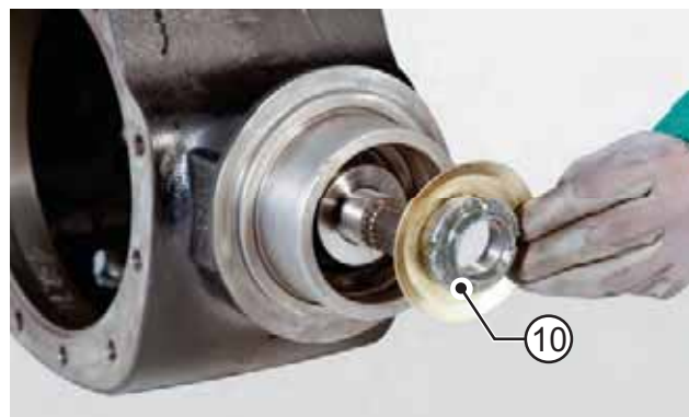
FIGURE 40: Apply tool T6 (See drawing T6 p. 71) and remove the ring nut (10).
