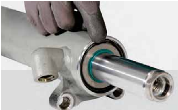
FIGURE 18: Introduce the stop ring and ensure that it sets in the seat of cylinder.
