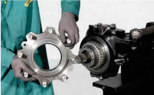
FIGURE 1: Remove the complete crown flange. For details, see PLANETARY REDUCTION GEAR p. 15.
