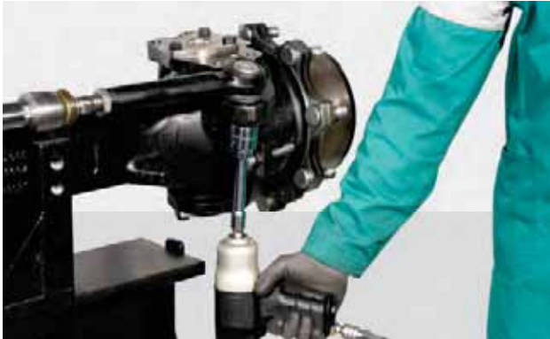
FIGURE 1: Remove the nuts (1) that lock the tie rods.
