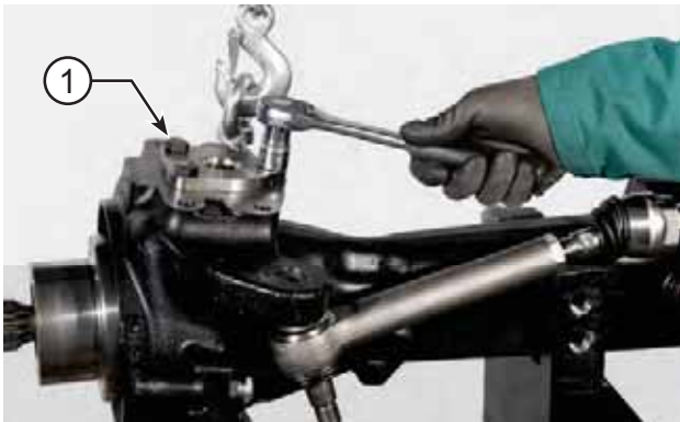
FIGURE 34: Loosen and remove the capscrews (1) from the kingpin (2).
