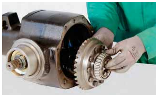
FIGURE 34: Install the whole differential unit.
