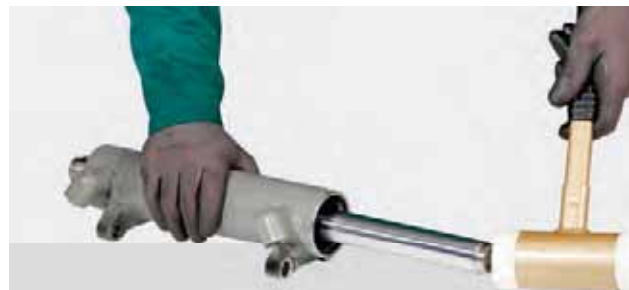
FIGURE 16: Push the piston into the cylinder using a plastic hammer.
