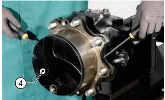
FIGURE 3: Disjoin the spider cover (4) from the hub by alternatively forcing a screwdriver into the appropriate slots.
