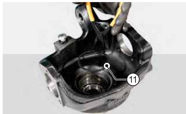
FIGURE 20: Fit the snap ring (11) of the bearing (10). Carefully check that snap ring (11) is completely inserted
