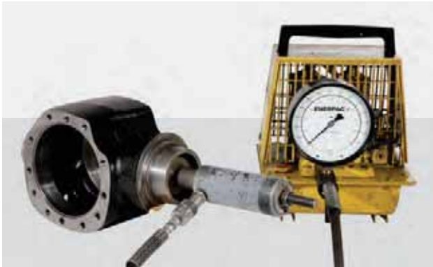
FIGURE 24: Connect the tension rod to the press and move the thrust block of the bearing (15, 17) into its seat. Disconnect the press and remove the tension rod.
