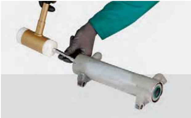
FIGURE 9: Continue hammering until the head is ejected from the cylinder.
