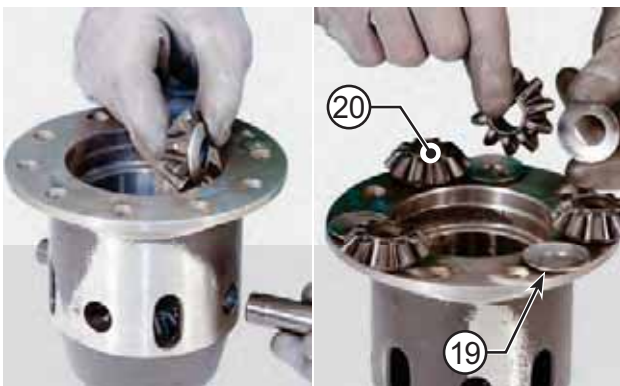
FIGURE 20: Remove the two half bolts (21), spherical washers (19) and satellite wheels (20).
