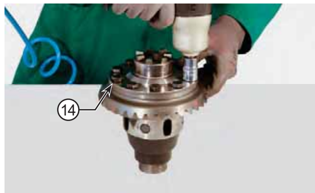
FIGURE 12: Remove the capscrews (14) of the crown (15). Note the position of assembly.
