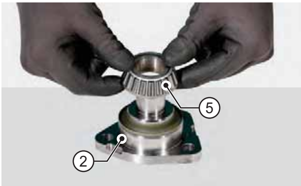
FIGURE 29: Install the bearing (5).
