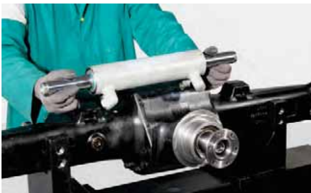
FIGURE 19: Fit the steering cylinder (5) into its seat.
