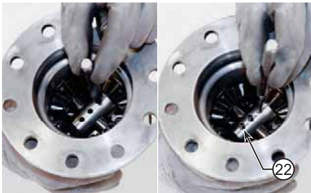
FIGURE 31: Bring the pin holes in line with the help of a pin-driver. Insert pins (22) to end of stroke.
