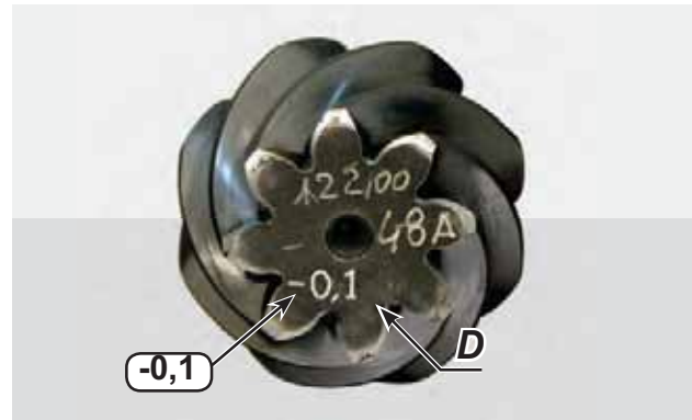
FIGURE 21: Check nominal dimension "D" as marked on the new pinion. Execute the calculation following the indicated formula to obtain the value of necessary shims. S = C - (D) Example: S = 1 - (+0,1) = 0,9 \text{ mm} S = 0,9 \text{ mm}
