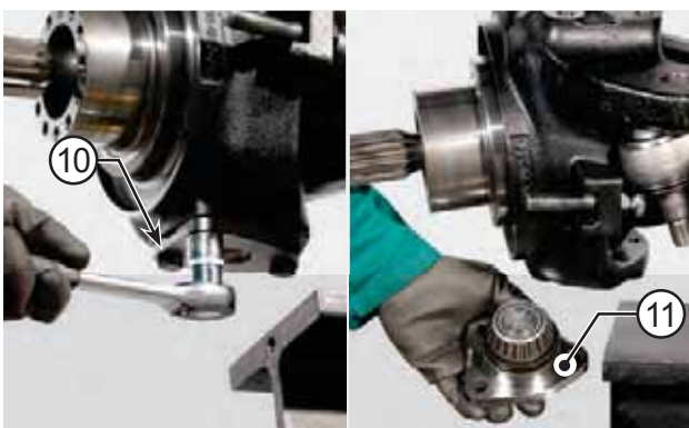
FIGURE 9: Loosen and remove the capscrews (10) from the kingpin (11). Remove the bottom kingpin (11).
