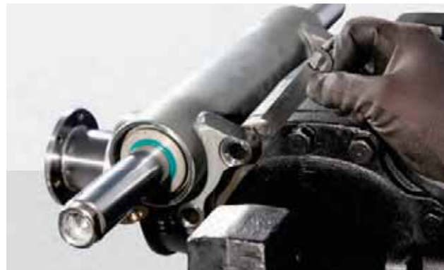
FIGURE 21: Install the predefined quote shim (6) (0,3 mm) in its seat, as shown in figure.
