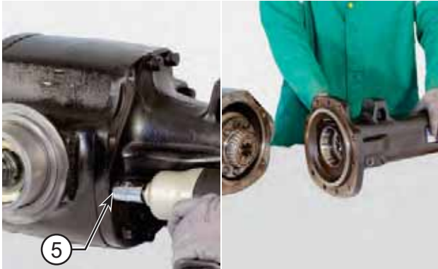
FIGURE 1: Connect a suitable lifting system. Loosen and remove the screws (5) securing the arm to the body. Remove the arm.
