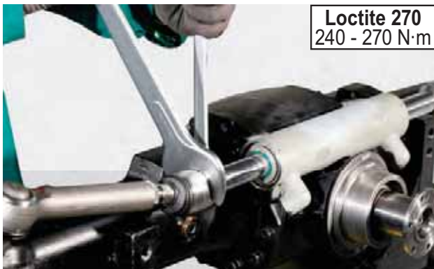
FIGURE 23: Apply LOCTITE 270 to the thread and connect the steering bars (3) by tightening the terminals onto the piston stem. Torque wrench setting: 240 - 270 N·m
