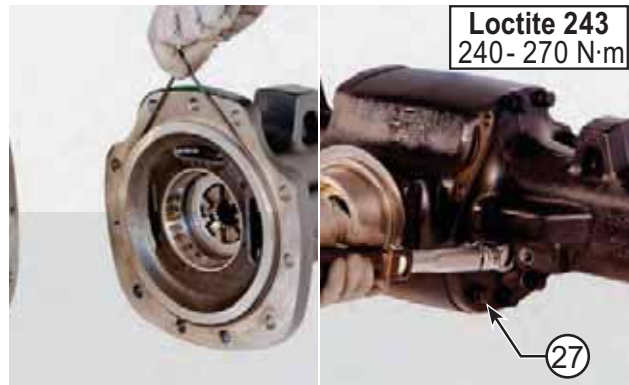
FIGURE 46: Insert a new o-ring on the centering diameter of the arm. Position the arm on the central body. Tighten nuts (27) in two stages, using the criss-cross method.
