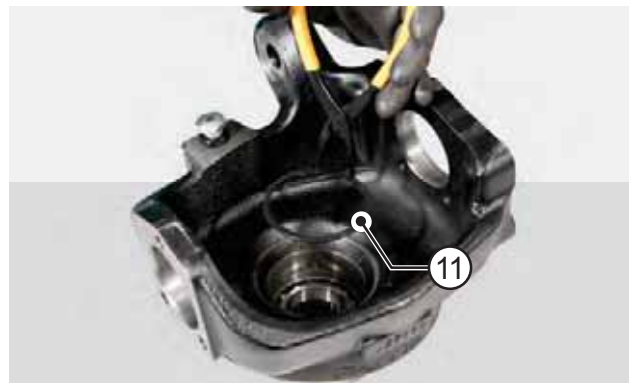
FIGURE 12: Remove the snap ring (11) from the steering knuckle.
