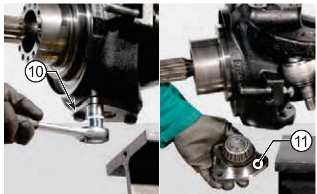
FIGURE 6: Loosen and remove the capscrews (6) from the kingpin (7). Remove the bottom kingpin (7).
