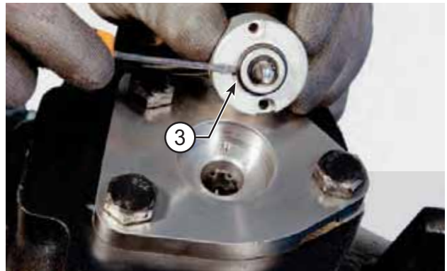
FIGURE 4: Remove the o-ring (3).
