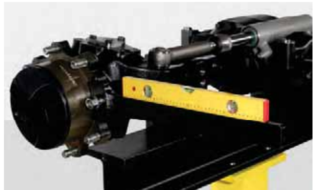
FIGURE 26: Apply tools T5 (See drawing T5 p. 70) to the hubs and lock them. Using a level, check that tools are perfectly flat.
