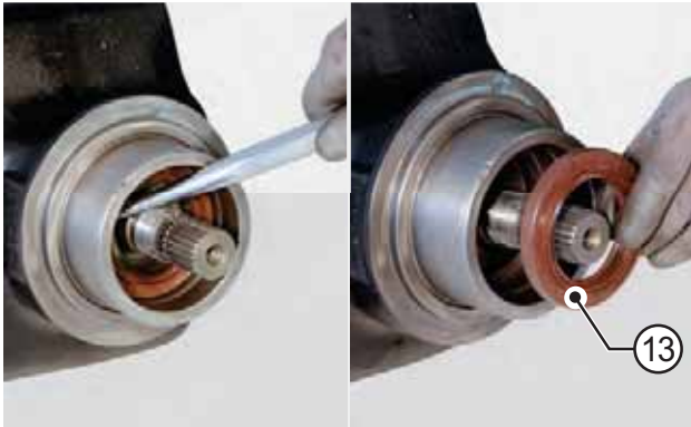
FIGURE 13: Using an internal extractor, remove the seal ring (13).
