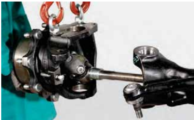
FIGURE 13: Tighten fully into the hole provided two double joint lifting eyes size M16, connect to suitable lifting gear and tighten. Pay attention not to damage the dust cover rings and the sealing rings. Install the steering knuckle.
