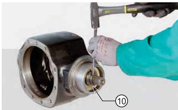
FIGURE 47: Caulk the ring nut (10).
