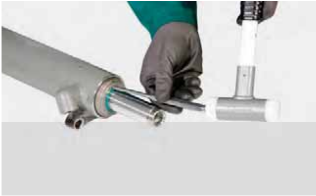
FIGURE 17: Lightly tap the cylinder head with a plastic hammer to push it inside the cylinder
