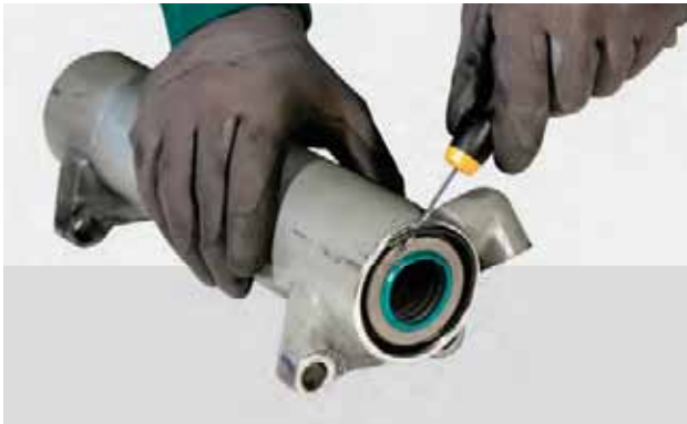
FIGURE 8: Remove the snap ring of the cylinder head.
