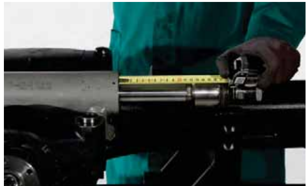
FIGURE 25: Center the piston by slowly moving it first in one direction then in the other and position it half way on the stroke.
