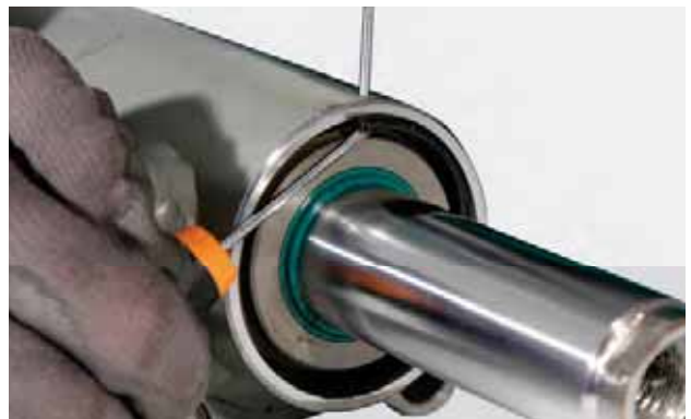
FIGURE 6: Remove the snap ring of the cylinder head.
