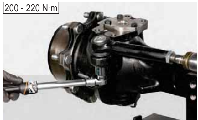
FIGURE 39: Install the tie rod nuts and lock into position using a torque wrench setting of 200 - 220 N·m.
