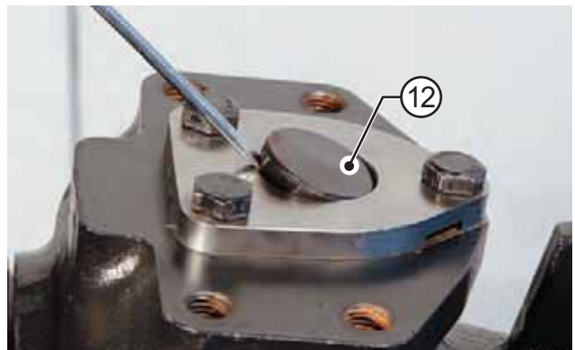
FIGURE 16: FOR MODELS WITHOUT SENSOR Remove the cap (12) before installing sensor.
