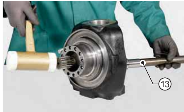
FIGURE 10: Remove the u-joint (13).
