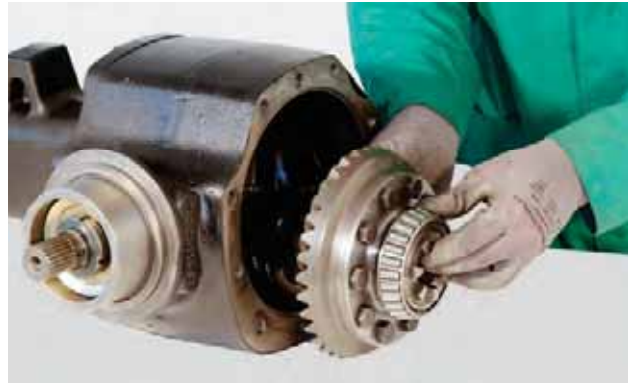
FIGURE 4: Extract the whole differential unit.
