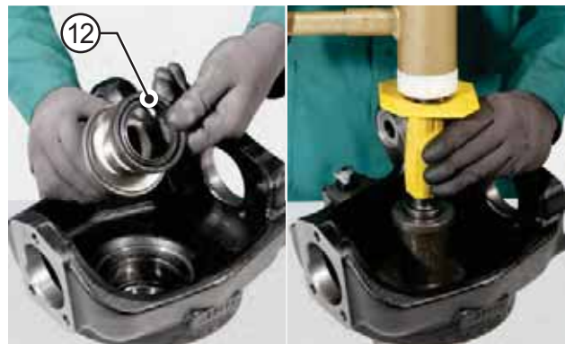
FIGURE 21: Lubricate the outer surface of the sealing ring (12) and assemble it into its position.
