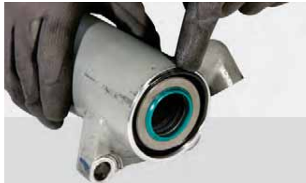
FIGURE 15: Apply grease to head seals, fit the head onto the piston and push it into the cylinder using a plastic hammer. Introduce the stop ring and ensure that it sets in the seat of cylinder.
