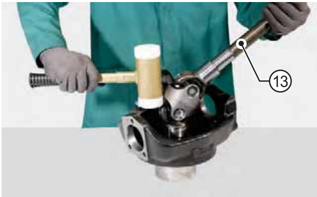
FIGURE 22: Lubricate the terminal of the u-joint (13) and install in the steering knuckle.
