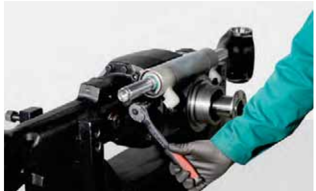
FIGURE 4: Remove the securing screws (4) from the steering cylinder.
