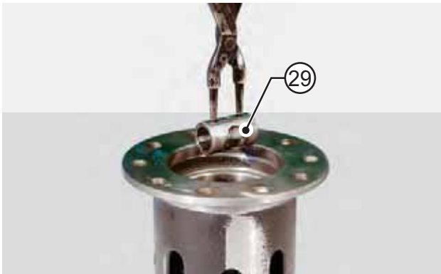
FIGURE 19: Remove the cross bolts (29).
