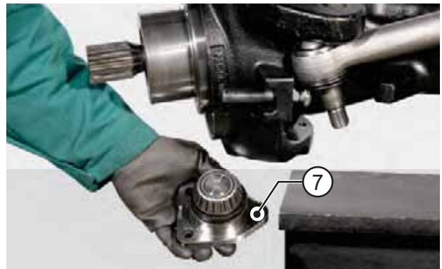
FIGURE 27: Grease generously the bearing (5) and the thrust block (5). Lubricate with OPTIMOIL grease the contact surfaces of the kingpin and steering knuckle.
