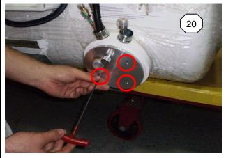
**30)** USING A PAIR OF CHANNEL LOCKS OR AN ADJUSTABLE WRENCH, REMOVE THE NUT FROM THE TANK RELIEF PORT AND SET ASIDE (IF EQUIPPED WITH PRV TUBE)
