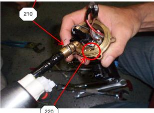
230) OBTAIN (2) SCREWS REMOVED IN STEP 140; ALIGN HOLES IN MOUNTING CLIP TO HOLES IN FUEL PUMP HOUSING; INSERT SCREWS THROUGH MOUNTING CLIP HOLES AND HAND TIGHTEN INTO FUEL PUMP HOUSING
