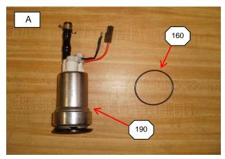
180) USING A FLAT TIP SCREWDRIVER, ALIGN AND SEAT O-RING
