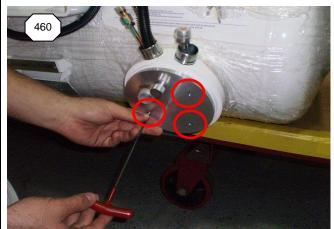
**460)** OBTAIN (3) COLLAR COVER SCREWS REMOVED IN STEP 20; INSERT SCREWS INTO HOLES IN LID; USING A 3mm ALLEN WRENCH, HAND TIGHTEN SCREWS INTO MULTIVALVE
