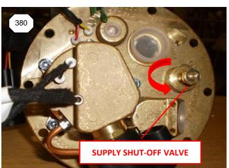
**380)** LOCATE SUPPLY SHUT-OFF VALVE ON MULTIVALVE: FULLY ROTATE KNOB 'COUNTER CLOCKWISE' TO OPEN SUPPLY VALVE
