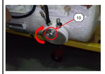
10) LOCATE MANUAL SUPPLY SHUT-OFF VALVE ON MULTIVALVE COLLAR COVER; ROTATE KNOB 'CLOCKWISE' UNTIL IT STOPS TO FULLY CLOSE SUPPLY VALVE
