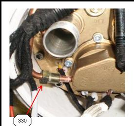
**330)** LOCATE FUEL PUMP SUPPLY LINE; HANDSTART FITTING ON LINE INTO HOUSING; USING AN 13mm WRENCH, FULLY TIGHTEN THE FITTING INTO THE HOUSING
