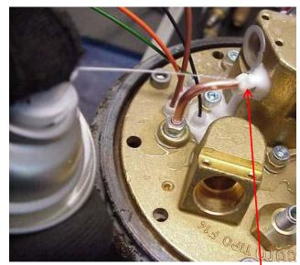
**400)** IF NO LEAKS ARE PRESENT, USE AN AIR HOSE AND NOZZLE TO REMOVE THE LEAK DETECTION SOLUTION FROM THE AREAS INSPECTED; LEAVE THE SUPPLY VALVE IN THE OPEN POSITION
