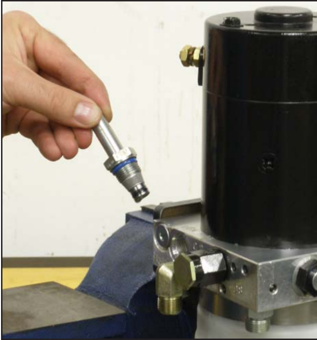
FIGURE 3-6 Remove "A" Valve. Clean by soaking cartridge in cleaning solvent.
