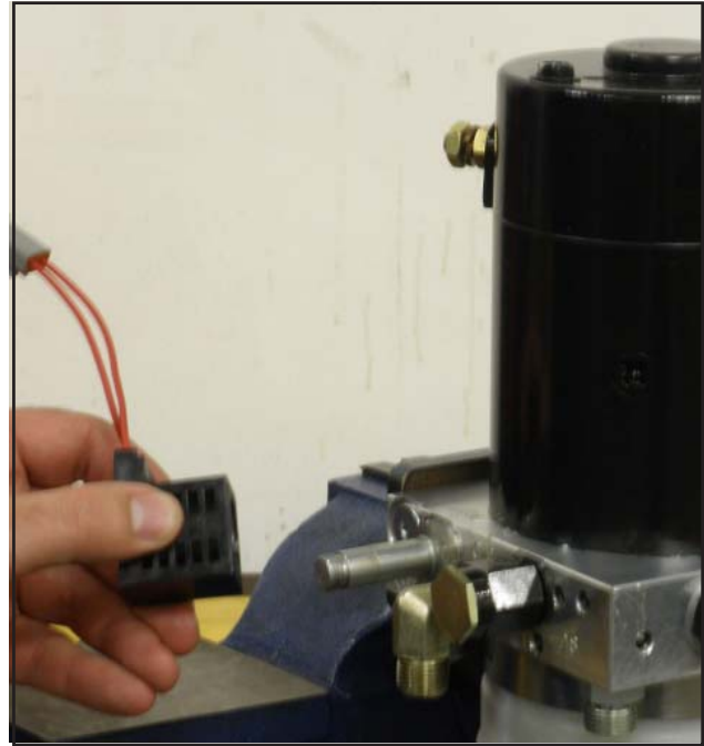
FIGURE 3-75 Re-install "A" Coil.
