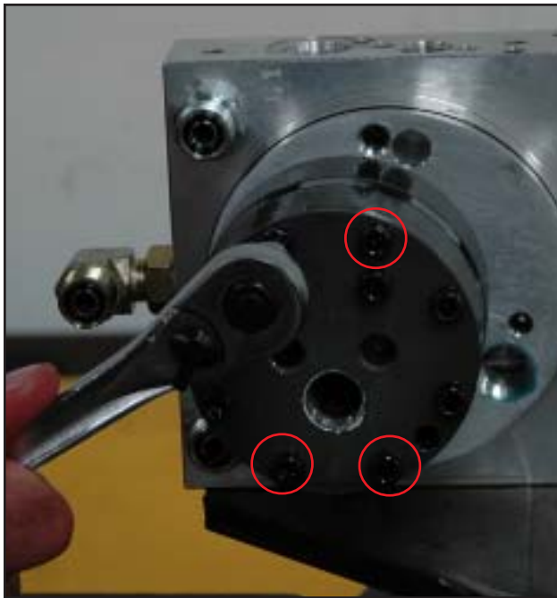
FIGURE 3-48 Torque all four pump mounting bolts to 100-125 in. lbs. be sure to torque in an even pattern.
