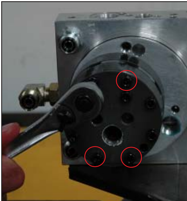
FIGURE 3-40 Use an allen wrench to loosen and remove the 4 bolts holding the pump to the base.
