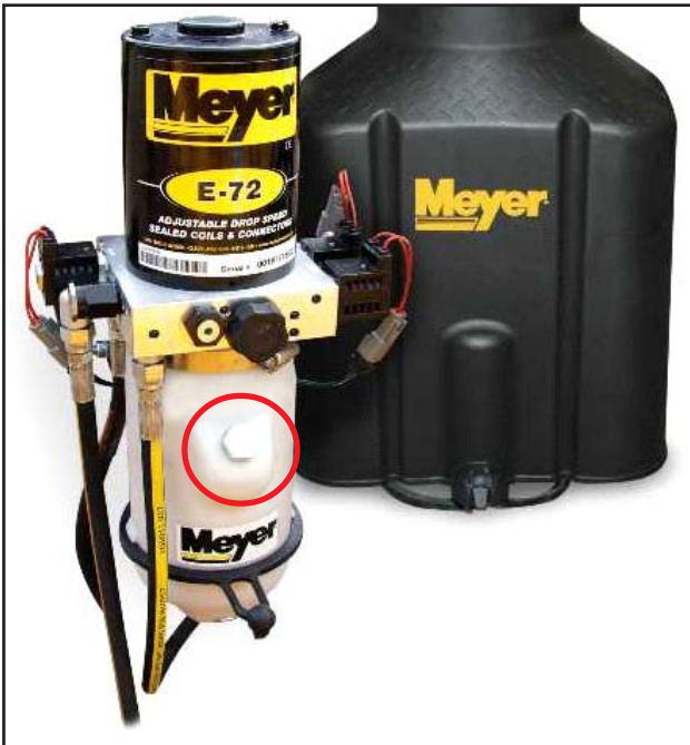
FIGURE 3-76 Fill Hydraulic Unit with Meyer M-1 Fluid. Flush out hoses, lift cylinder and both angle cylinders before operating plow.
