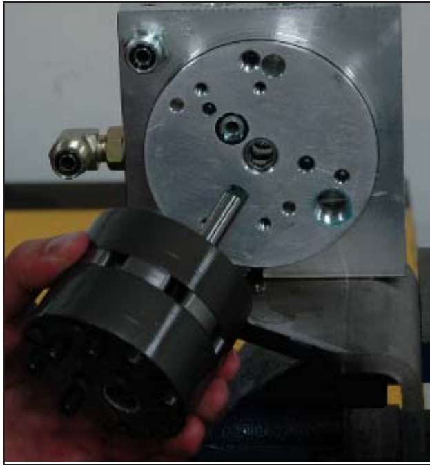
FIGURE 3-46 Replace pump to base o-ring and re-install pump.
