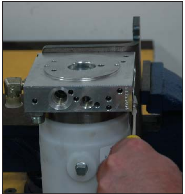
FIGURE 3-33 Use a screwdriver to loosen reservoir clamp and remove clamp.
