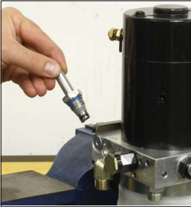
FIGURE 3-74 Re-install "A" Valve.
