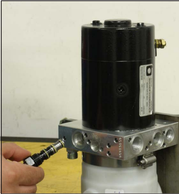
FIGURE 3-66 Re-install Pilot Check Valve Assembly.
