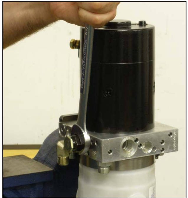
FIGURE 3-65 Turn in allen screw to raise and out to lower pressure. Valve should open when 3000 PSI is attained and allows the plow to angle. This valve enables the plow to absorb impacts.
