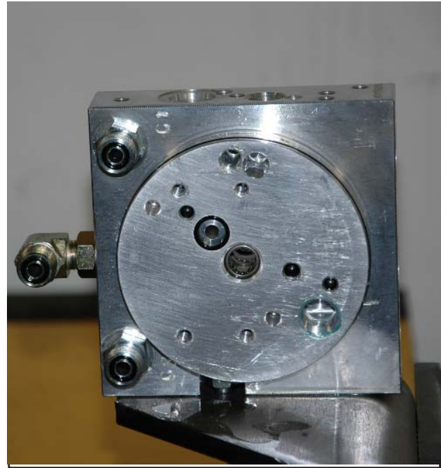
FIGURE 3-43 Clean base with cleaning solvents and inspect pump shaft bearing. If bad replace the base.
