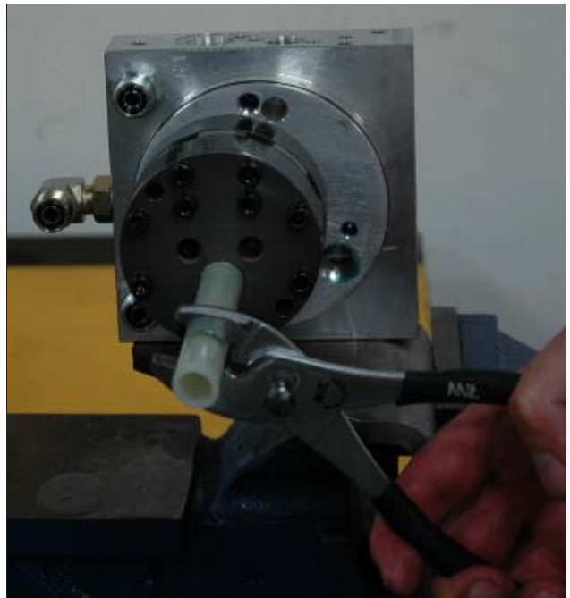
FIGURE 3-49 Re-install oil pick-up tube to pump. Do not overtighten or use any thread sealant.
