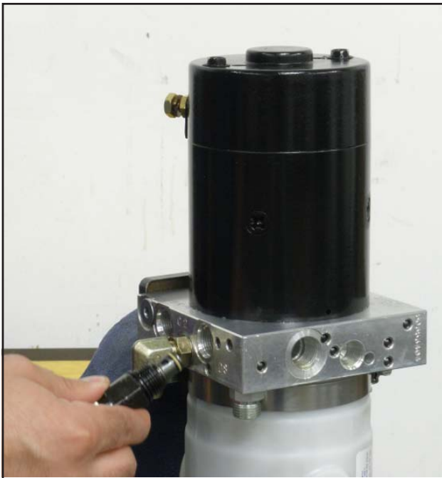
FIGURE 3-64 Re-install Cross-over relief valve. Tighten Cross-over relief valve. Pressure is adjustable and should be set to 3000 PSI. In order to adjust set a guage in angle ram and apply pressure to angle system at plow.
