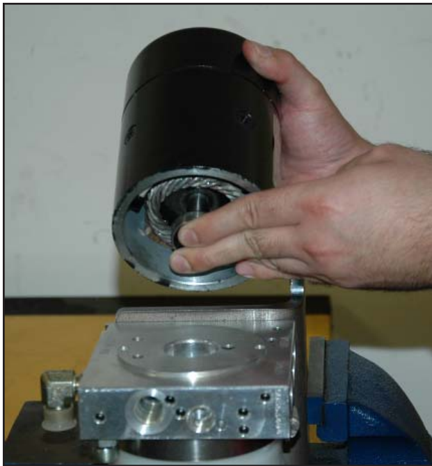
FIGURE 3-32 Hold the motor parts together while removing it from the pump base.
