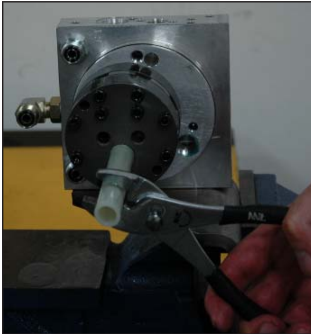
FIGURE 3-38 Carefully loosen and remove plastic oil pick up tube.
