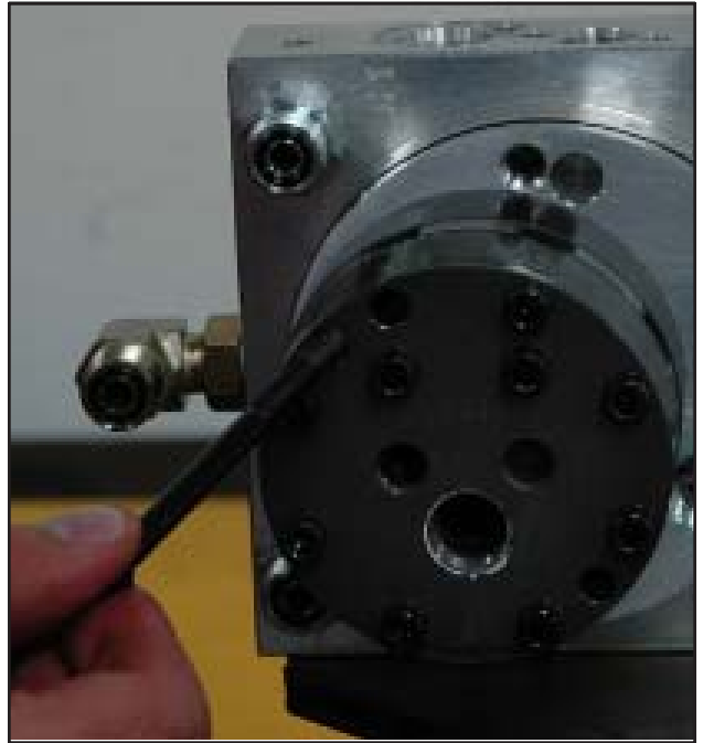
FIGURE 3-47 Attach pump to base with 4 allen head bolts.
