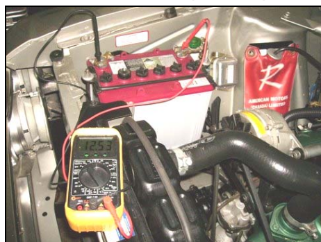
In this illustration, with engine off, the meter reads 12.53
