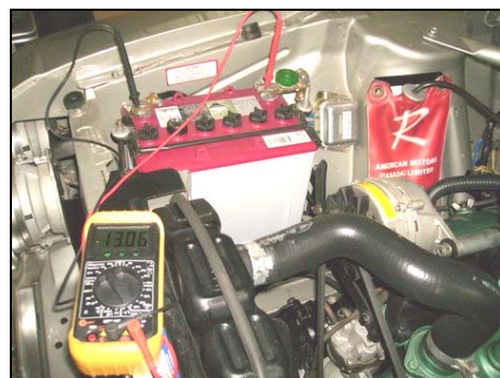
Back at normal idle speed, the meter reads 13.06
