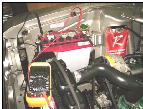
Here, the engine is running at 1500 r.p.m., & it reads 14.05
