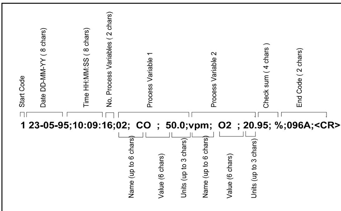
Figure 5.2 Format of serial output data frame
