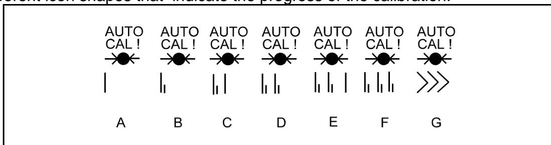
Figure 4.2 Screen icons indicating autocalibration progress
