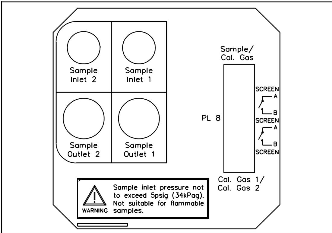
Figure 2.10 Sample gland plate with external auto calibration
