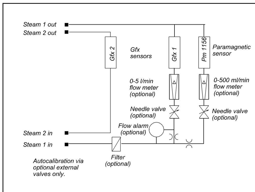
Figure 2.12 Typical dual stream, dual Gfx configuration
