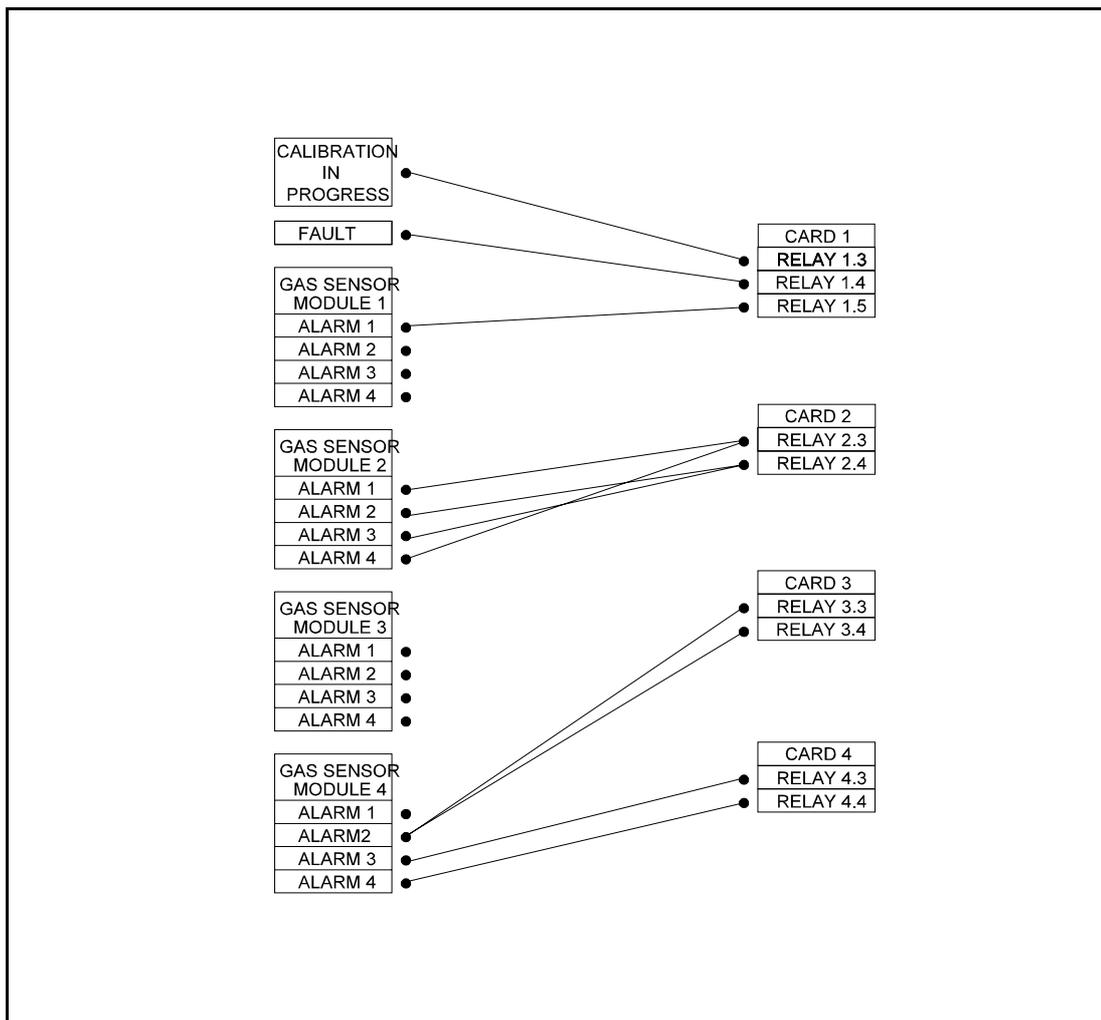
Figure 5.1 Allocation of relays
