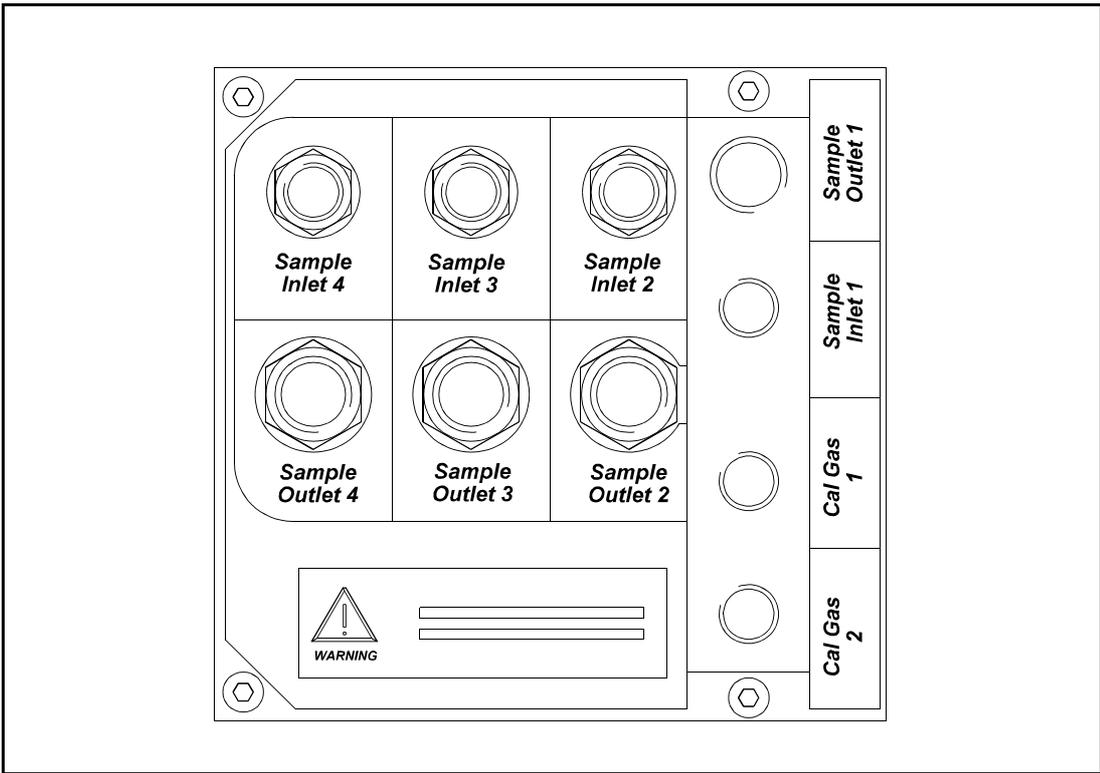
Figure 2.9 Sample gland plate with internal auto calibration
