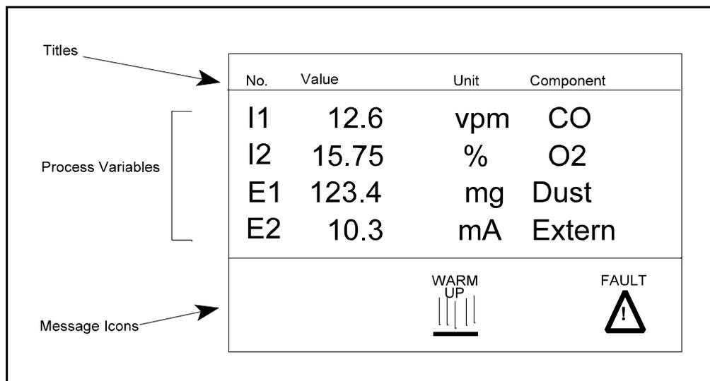
Figure 1.2 Xentra measurement display
