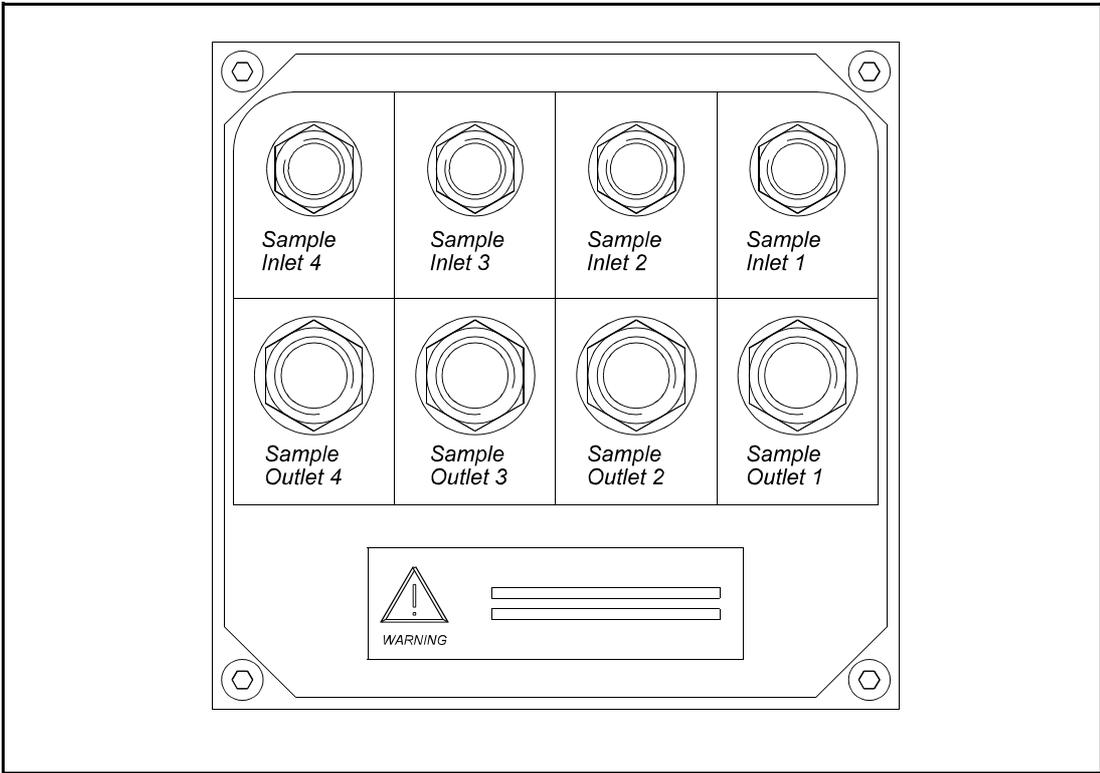
Figure 2.8 Sample gland plate without auto calibration
