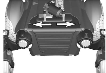
*Figure 115. Knobs holding the front cover.*
