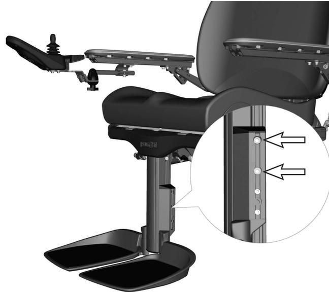
*Figure 18. The height of the foot plates is secured using the outer locking screws*
