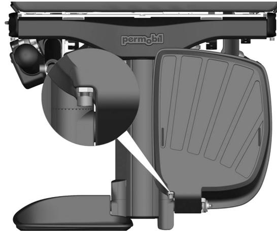
*Figure 19. The angle of the foot plates can be adjusted using a screw locked with a lock nut.*
