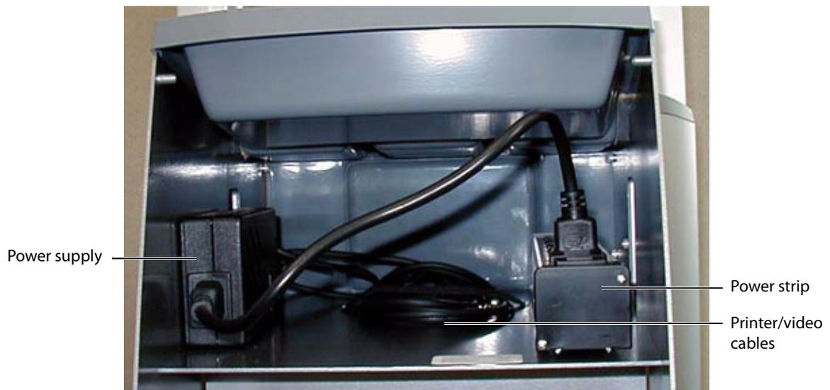
Figure 9.14 Mobile Docking System Power Supply
