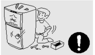
In case of unstable power supply or during cleaning, it is required to pull out the power plug, and to wait at least 5 minutes for switching on it again to prevent damaging its compressor by continuous starting.
