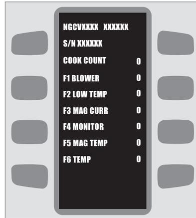
FIGURE 3: Fault Display
