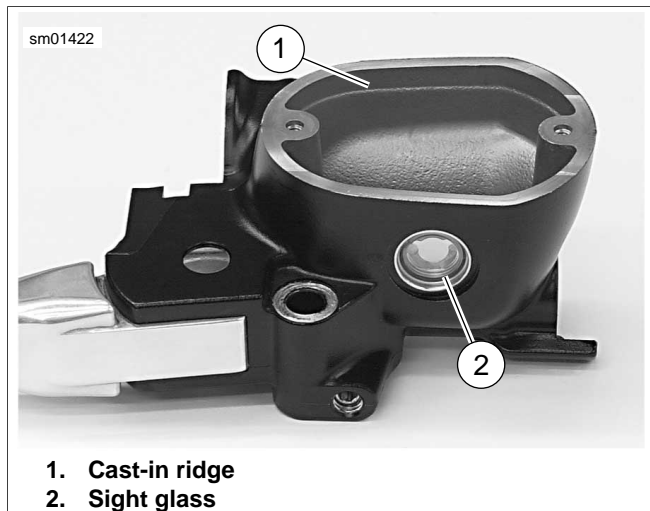
Figure 1-11. Filling Front Master Cylinder Reservoir
