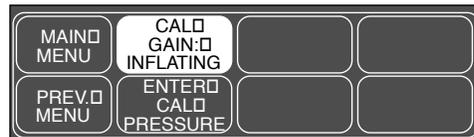
4. The pump shuts off at about 250 mmHg, and the pressure drops slowly to about 240 mmHg before stabilizing. The second line of text on the CAL GAIN menu item changes from INFLATING back to HOLDING. If the pressure continues to drop at a rate of 4 mmHg/min or more, there is a leak in the NBP plumbing. If there is a leak in the NBP plumbing, repair it and restart this calibration procedure.
