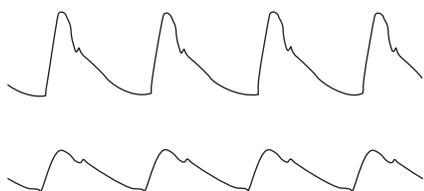
1. If the calibration pulses were not correct, test the patient simulator using a working monitor. If the patient simulator is functioning as designed, you may need to replace the acquisition PCB.
