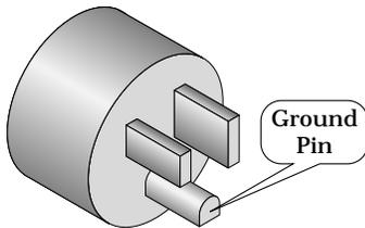
Listed below are two methods for checking the ground (earth) integrity, "Ground Continuity Test" and "Impedance of Protective Earth Connection." These tests determine whether the device's exposed metal and power inlet's earth (ground) connection has a power ground fault condition.
