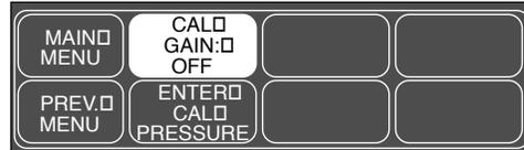
3. Rotate the Trim Knob control to highlight START, and then press the Trim Knob control to select it. The second line of text on the CAL GAIN menu item changes from OFF to INFLATING. Then, the monitor starts pumping up the pressure bulb or cuff – the audible whirring sound of the NBP pump motors occurs and an increase in displayed pressures on both the monitor and the manometer can be observed.
