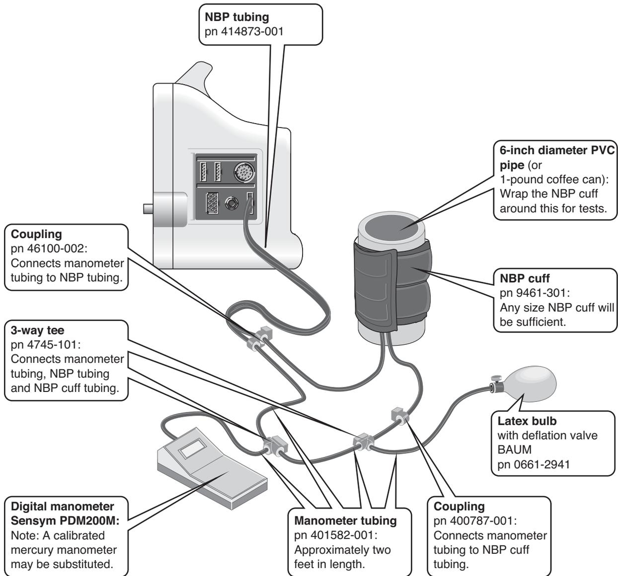
7. The service menus should appear on the monitor display. These next steps guide you through the service menus associated with checking NBP calibration and checking for leaks. If desired test results are not obtained, NBP calibration is necessary.
