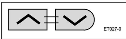
2. Set the Treated Water Capacity. Using the **Set Up** or **Set Down** buttons, set the amount of treated water to flow through the unit before a regeneration is required.
