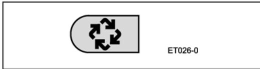
Push the **Extra Regeneration** button to start an extra regeneration tonight. Push and hold the **Extra Regeneration** button for 5 seconds to start an **Extra Regeneration** immediately.
