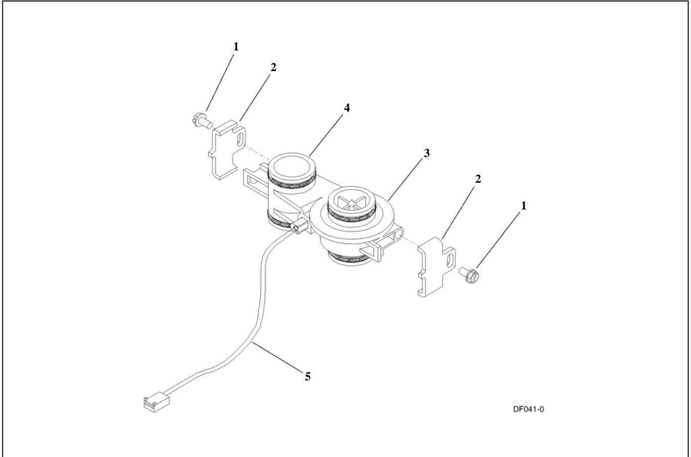
Figure 17: 3/4" Turbine Meter Assembly
