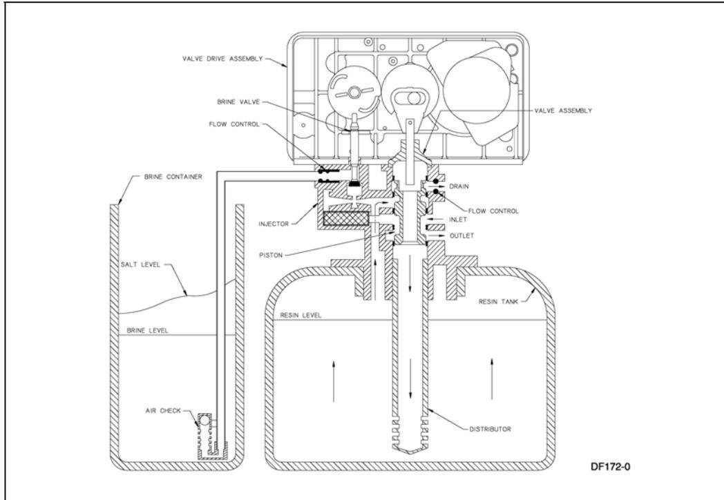
Figure 11: Second Backwash Position (Double Backwash Units Only)
