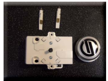
Loosen the screws as shown to remove the rotating switch
