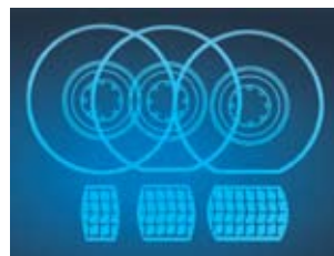
Lower pressure results in larger tire footprint.
