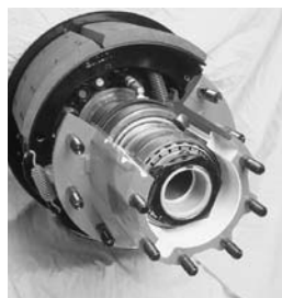
Spicer TPCS features integrated drive axle air seals with no vulnerable, external lines to avoid costly repairs and downtime. All rotating seals are internally mounted for reliable operation.
