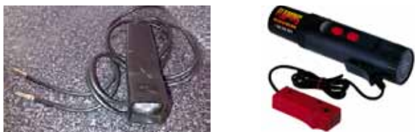
Old neon timing light (l) vs. new Flaming River self-powered one (r).
