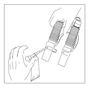
Your 2001 MARS Fork requires periodic maintenance, cleaning, and inspection. Moisture and contamination may build up inside the fork depending on the severity of riding conditions. To maintain top performance, it is recommended that the fork be periodically disassembled, cleaned, dried and re-greased using Prep-M grease. See Figure 6.
