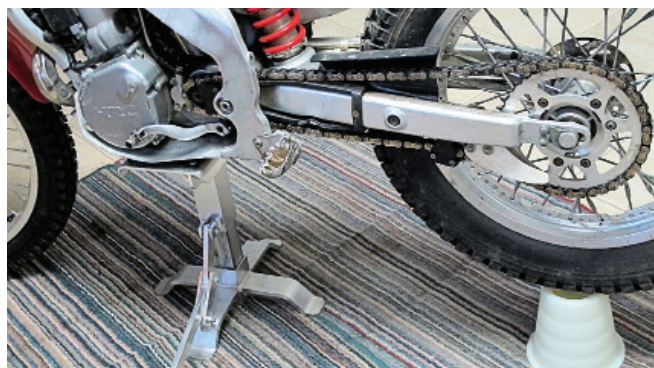
For rear suspension service, the bike must be supported from under the engine, frame or sub-frame; the swingarm cannot bear weight. It will, however, need to be supported to relieve extension pressure on the shock and linkage, thereby allowing their removal. Ugly old rugs come in handy when playing mechanic in the kitchen.
