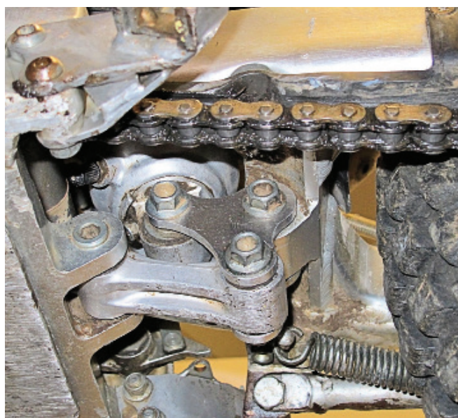
This linkage is extremely compact to save weight and stay tucked out of harm's way—relatively speaking. It has actually taken quite a bit of abuse on this trials bike. Linkage systems can include more segments, but the principles involved remain the same.
