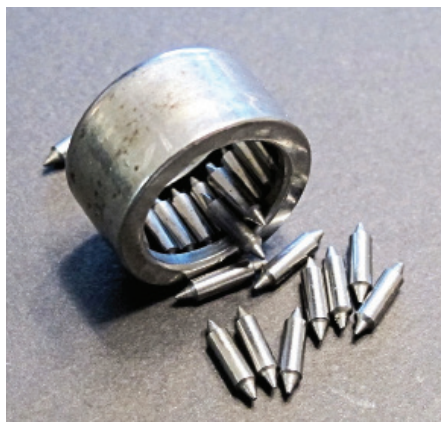
This old bearing was in pretty good shape. Stripped of its grease by solvent, it released its needles readily. Note that each needle has a small cone on each end that is normally retained by the race's edge.
