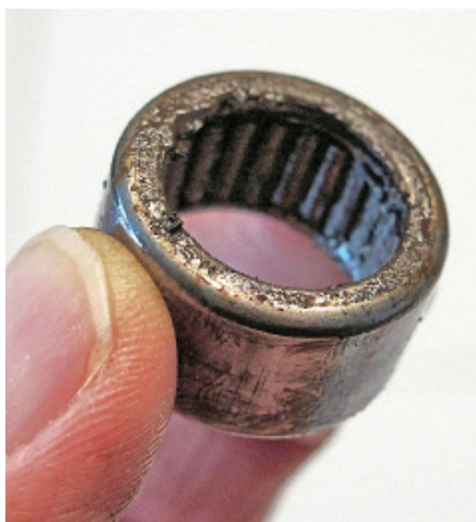
This old bearing was packed with mud and rust; its needles barely turned at all.
