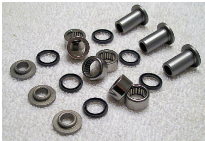
Ironically, All-Balls makes needle bearings, too. This kit includes all the bushings, seals and bearings shown here for our example bike, along with the lower shock joint and its seals (not shown), which we deemed unnecessary at this point and saved for the future.
