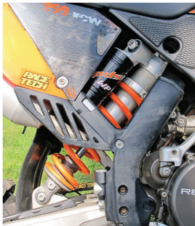
This linkage-less rear suspension is worlds simpler and easier to maintain, but its PDS (Progressive Damping System) only approximates the progressive feel of a linkage. KTM owners take heed: The heim joint at the lower end of your shock should NEVER be lubricated; its Teflon surface will be destroyed by the resulting grit accumulation.
