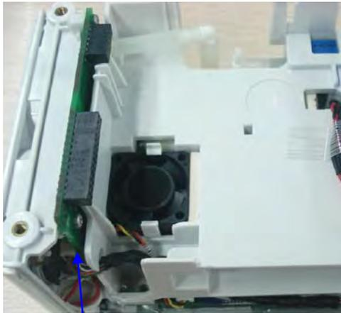
Withdraw the analog out cable from the hole beside the fan
