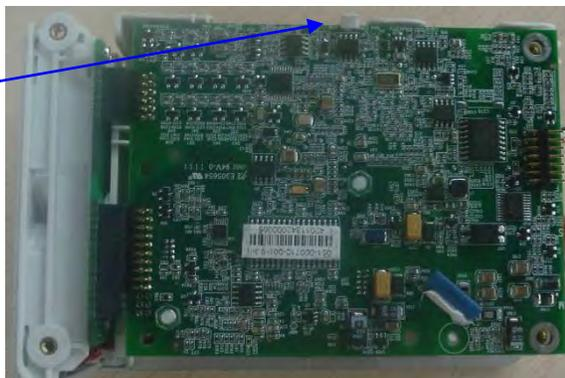
4. Unscrew the two M3×4 screws that secure the SpO2 board, and then remove the SpO2 board.
