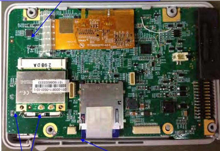
Loosen the latch and then remove the Wi-Fi module PCBA
