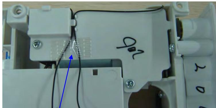
Separate the two cables and use tape to secure the cables onto the main frame
