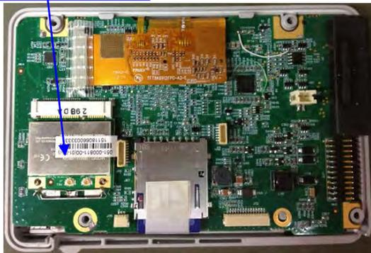
5. Insert the antenna plugs into the Wi-Fi sockets (socket on the left for the cable on the left and socket on the right for the cable on the right). Secure the antenna plug with tape.
