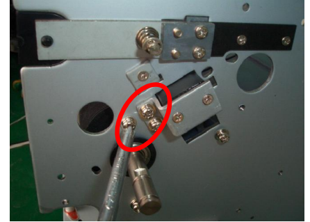
Screw off the four screws fixing the Front Lower Transfer Mechanism on the right and left sides.
