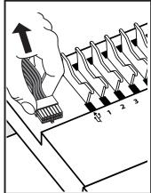
Unwind and remove the existing USB cables from drawer.
