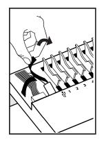
Unplug the USB and DC power cables (push up on the lever under the DC connector to release). The drawer can now be removed.
