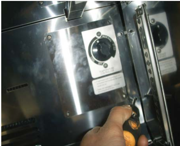
D. Disassemble the evaporator duct
