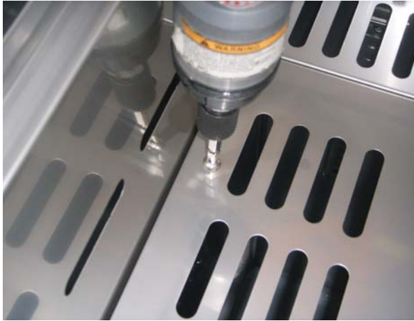
C. Disassemble the pan duct middle
