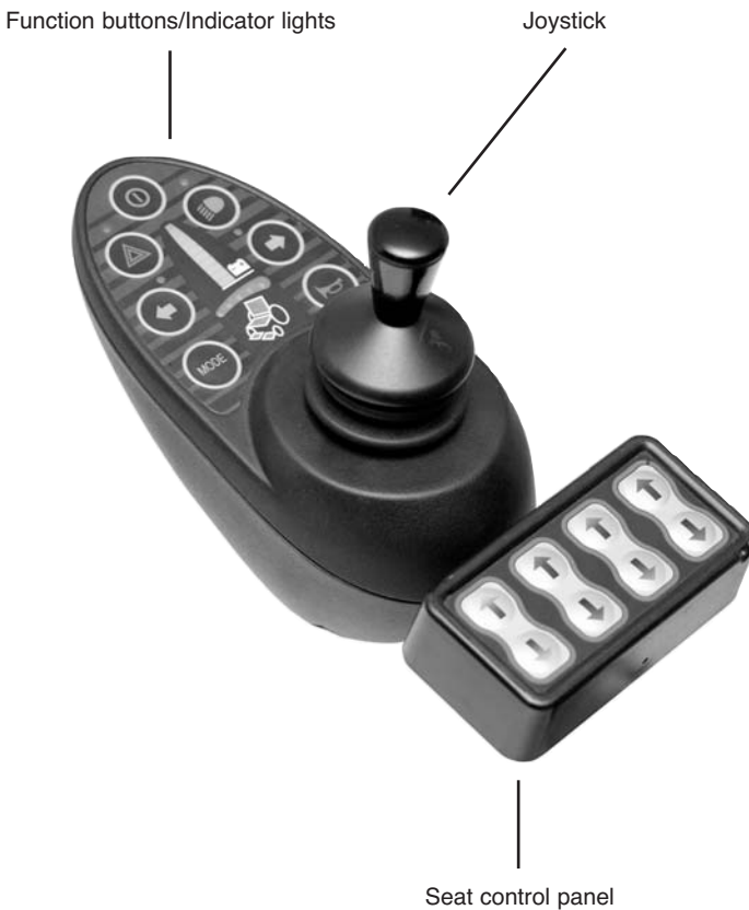
Pilot + control panel overview
