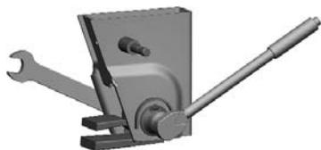
Marking for angle tightening
