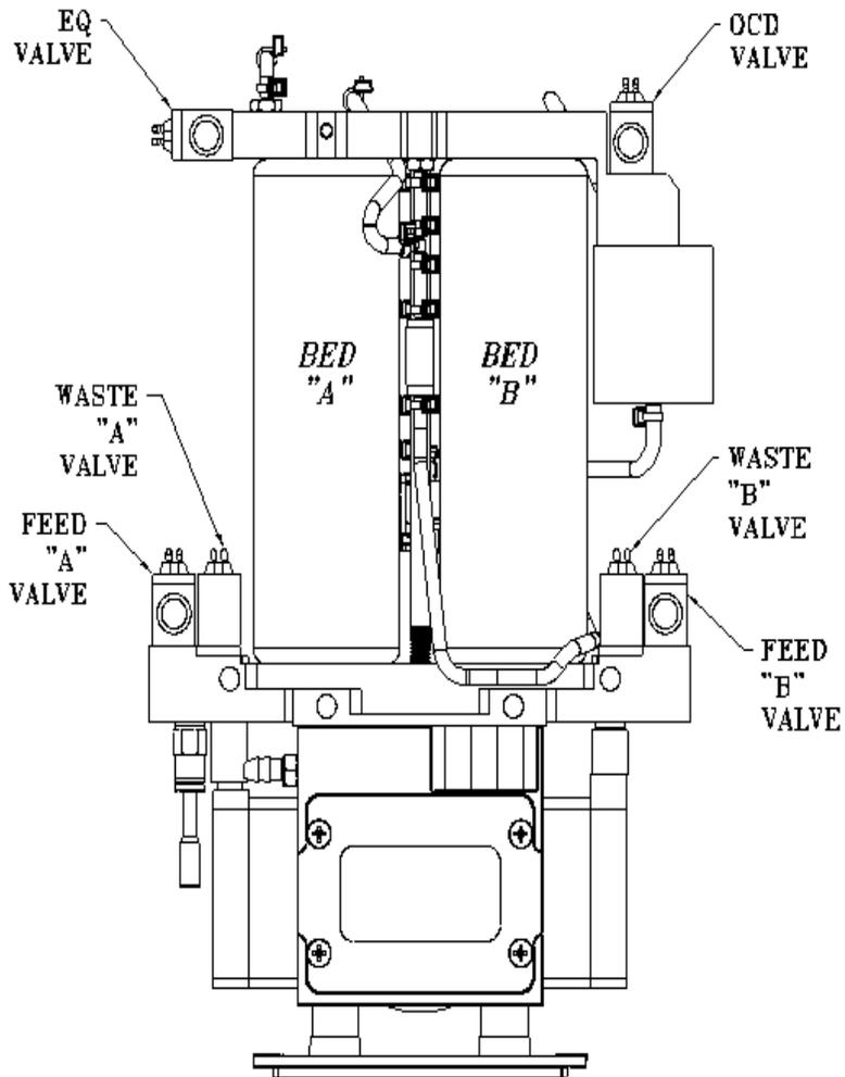
Figure A.4: PSA Assembly Feed / Waste
