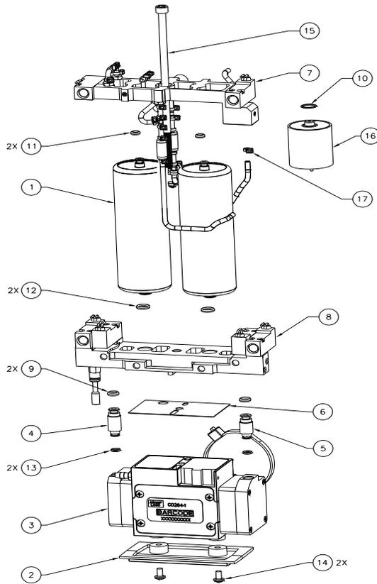
Figure A.3: PSA Assembly – Product Manifold
