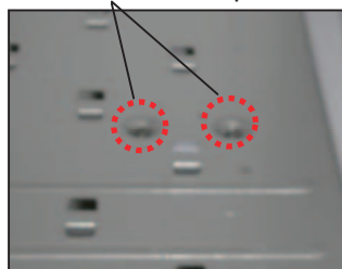
<Temp. sensor mounts on lowest shelf>
