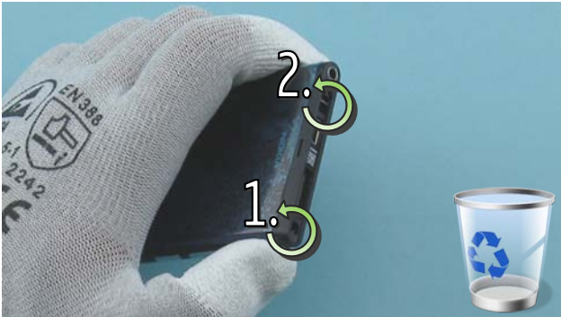
7) Unscrew the two Torx+ size 4 screws. Do not use them again. Discard them.
