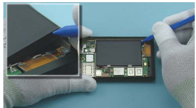
24) Use the sharp end of the SS-93 to lift up the BATTERY.
