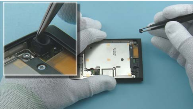
19) Remove the FRONT CAMERA BOOT with the tweezers.
