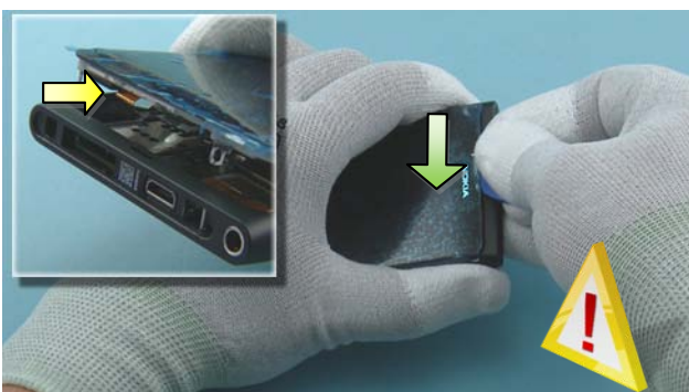
11) Slide the SRT-6 along the top side of the phone, between the DISPLAY ASSEMBLY and the PLASTIC BODY. Be careful not to damage the shown flex located halfway the top side.
