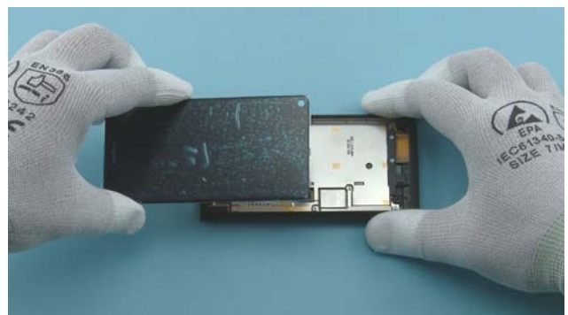
18) Remove the DISPLAY ASSEMBLY.
