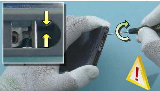
9) Insert a flathead screwdriver in the shown hole on the top side of the phone. Twist the screwdriver so that the DISPLAY ASSEMBLY slightly rises out of the PLASTIC BODY. Be careful not to damage the PLASTIC BODY.
