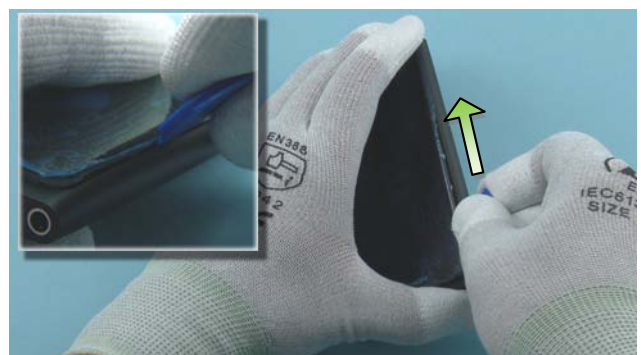
12) Use the SRT-6 to open the left side of the DISPLAY ASSEMBLY.
