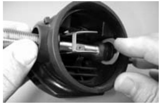
Fig. 30 – Installing Retaining Clip
