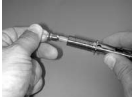
Fig. 10 – Removal of Adjustable Orifice
