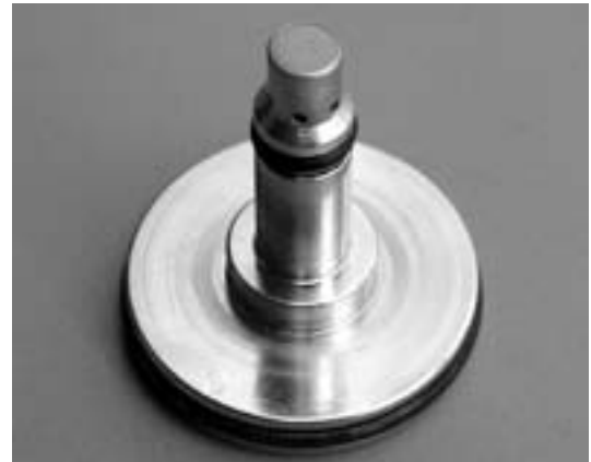
Fig. 12 – HP Seat Installation
