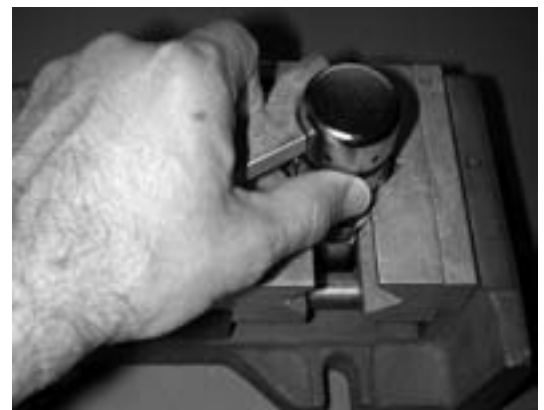
Fig. 1 – Loosening the Piston Cap
