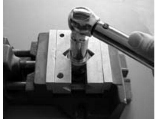
Fig. 15 – Torquing DIN Housing
