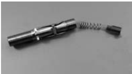
Fig. 9 – Removal of LP Spring
