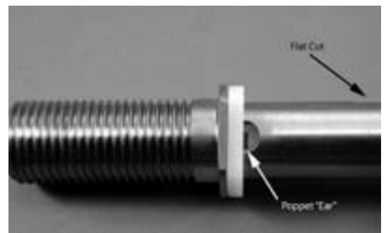
Fig. 25 – Poppet Correctly Installed
