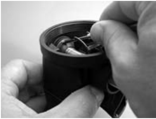
Fig. 7 – Removal of Retaining Clip
