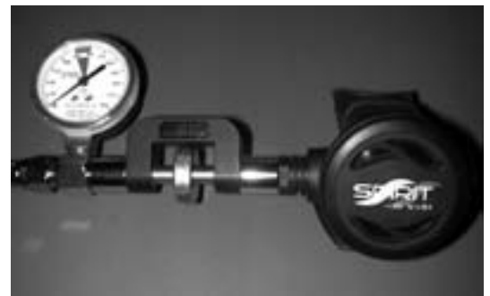
Fig. 35 – Inline Adjustment Tool w/ IP Gauge
