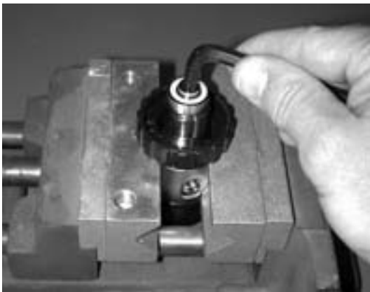
Fig. 4 – Removal of DIN Retainer
