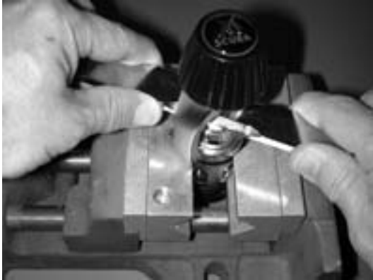
Fig. 2 – Loosening the Yoke Retainer
