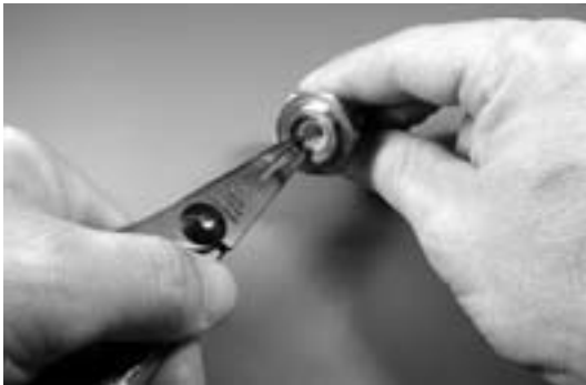
Fig. 3 – Removal of Filter Retaining Ring
