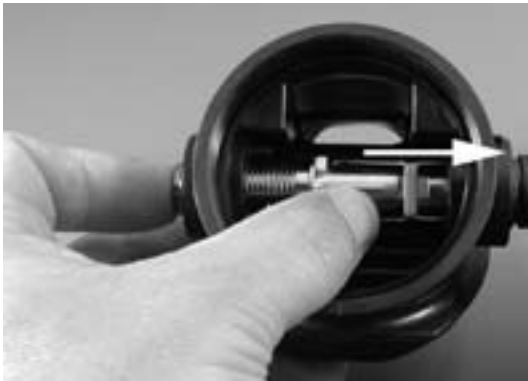
Fig. 8 – Removal of Valve Assembly
