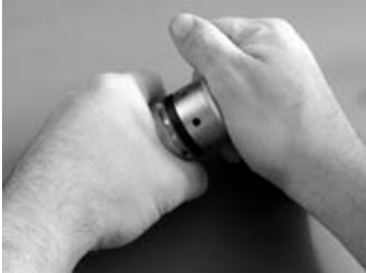
Fig. 13 – Installing Piston Cap
