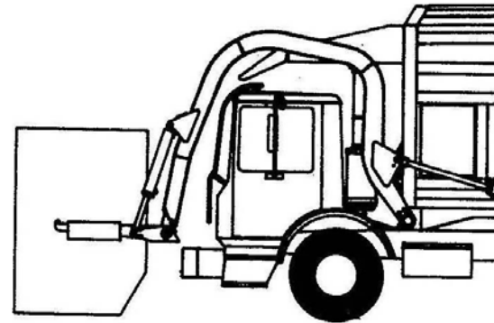
Figure 45. Rotate Container Back Before Lowering
