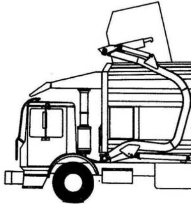
Figure 44. Dump Container into Hopper
