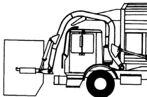
Figure 42. Fully Insert Forks into Container Pick-up Sleeves
