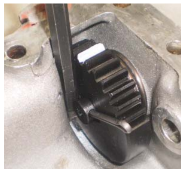
FIGURE 5; COTTER PIN INSTALL
