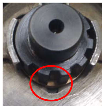
FIGURE 8; BACKING PLATE TIMING
