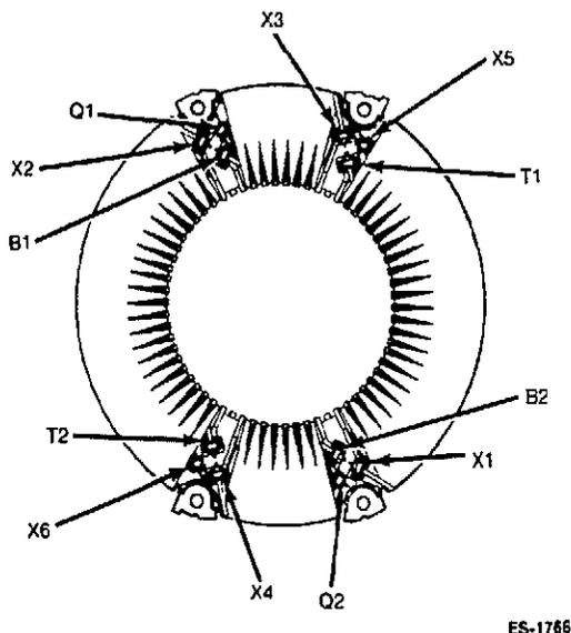
FIGURE 8-12. STATOR ASSEMBLY
