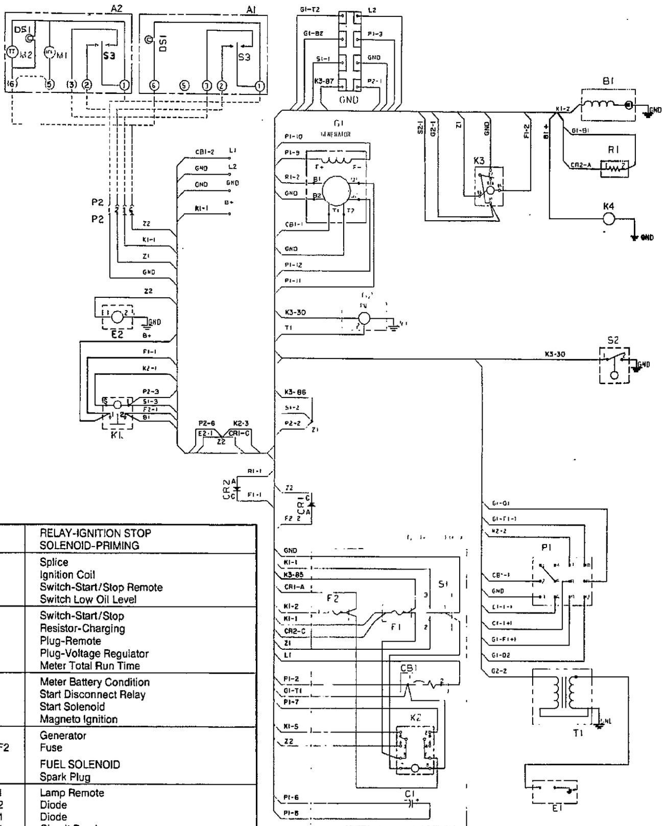
FIGURE 8-2. LPG GENERATOR SET WIRING DIAGRAM - 60 HERTZ
