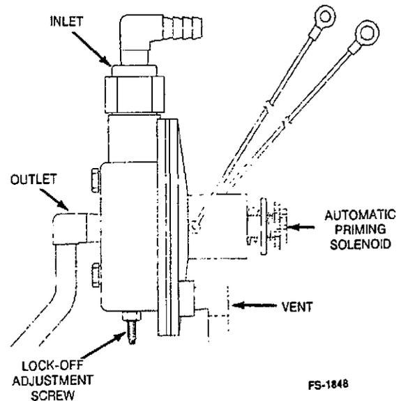
FIGURE 6-17. DEMAND REGULATOR WITH AUTOMATIC PRIMING SOLENOID
