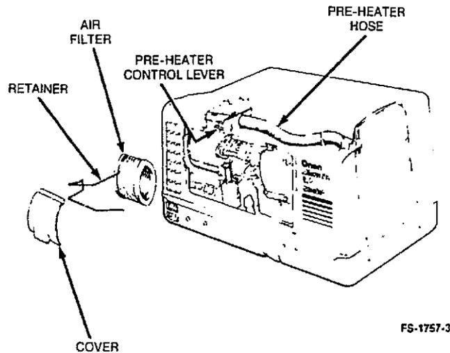
**FIGURE 6-7. AIR FILTER AND PREHEATER ASSEMBLY**
