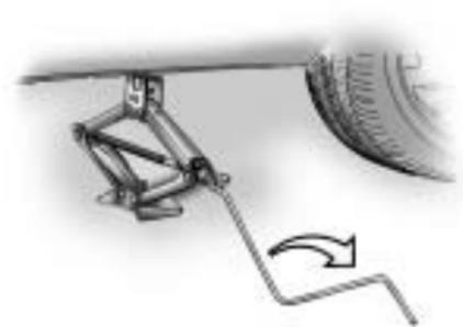
7. Turn the jack handle clockwise. Raise the vehicle far enough off the ground so there is enough room for the compact spare tire to fit underneath the wheel well.
