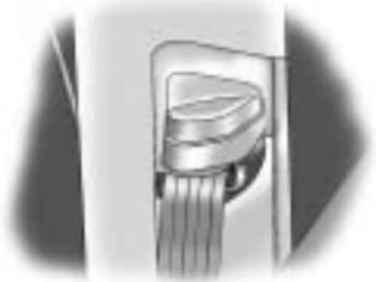
Push down on the release button and move the height adjuster to the desired position. The adjuster can be moved up by pushing on the front of the height adjuster.
