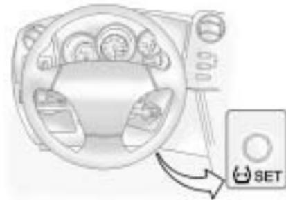
5. Press and hold the tire pressure warning reset switch until the tire pressure warning light flashes slowly on/off three times. Wait for a few minutes with the ignition in ON/RUN, and then turn the ignition to ACC/ACCESSORY or LOCK/OFF.
