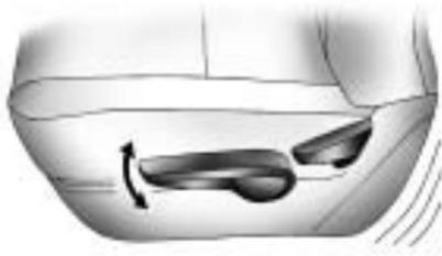
The driver seat height adjuster is located on the outboard side of the seat. To raise or lower the seat, pull up or push down on the lever repeatedly until the seat is at the desired height.
