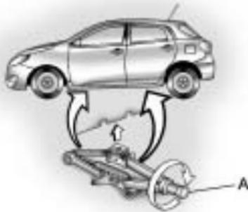
6. Position the jack and raise the jack lift head to fit over the car flange between the two notches.
