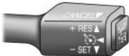
For vehicles with cruise control, the lever is located on the right side of the steering wheel.
