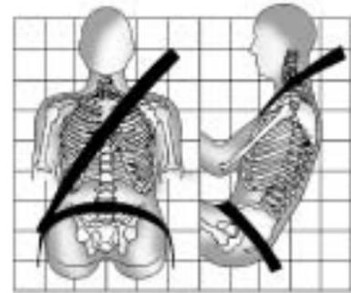
Sit up straight and always keep your feet on the floor in front of you. The lap part of the belt should be worn low and snug on the hips, just touching the thighs. In a crash, this applies force to the strong pelvic bones and you would be less likely to slide under the lap belt.
