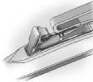
3. Slide the new wiper assembly into place.
