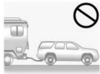
Do not tow the vehicle from the rear. The vehicle could be badly damaged and the repairs would not be covered by the warranty.
