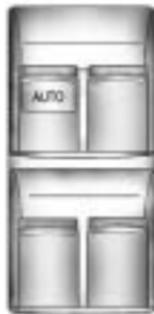
On vehicles with this feature, the power windows only work when the ignition is turned to ON/RUN or in Retained Accessory Power (RAP). See *Retained Accessory Power (RAP)* on page 8-18.
