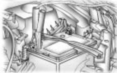
6. Connect the red positive (+) cable to the positive (+) terminal of the dead battery. Use a remote positive (+) terminal if the vehicle has one.
