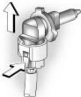
3. Unplug the connector while pressing down on the release tab.
