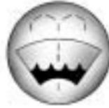
Open the cap with the washer symbol on it. Add washer fluid until the holes of the dipstick are filled between the LOW (B) and NORMAL (A). See *Engine Compartment Overview* on page 9-6 for reservoir location.
