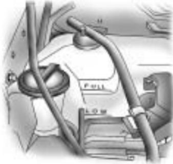
If you need more coolant, add the proper DEX-COOL<sup>®</sup> coolant mixture at the coolant recovery tank, but be careful not to spill it.
