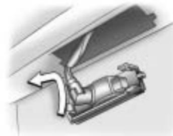
2. Turn the bulb socket counterclockwise to remove it from the license plate assembly.
