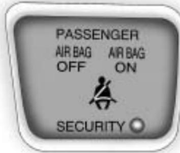
The words ON and OFF will be visible during the system check. When the system check is complete, either the word ON or the word
