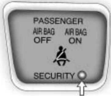
The security light is in the center of the instrument panel.
