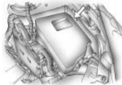
This engine compartment fuse block is located in the engine compartment on the driver side of the vehicle near the air cleaner. See *Engine Compartment Overview* on page 9-6.
