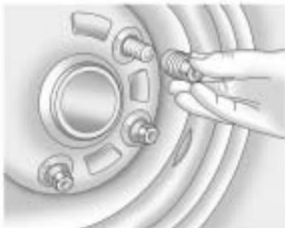
8. Remove the wheel nuts and the flat tire.
