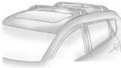
**Notice:** Loading cargo on the roof rack that weighs more than 75 kg (165 lbs) or hangs over the rear or sides of the vehicle may damage the vehicle. Load cargo so that it rests evenly between the crossrails, making sure to fasten cargo securely.
