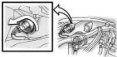
2. Turn the bulb socket counterclockwise and pull it out of the lamp assembly.
