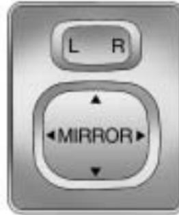
The controls are located to the left of the steering wheel on the instrument panel. The vehicle must be in ON/RUN or ACC/ACCESSORY to adjust the mirrors.
