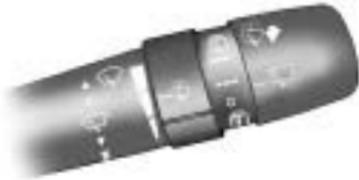
The windshield wiper/washer lever is located on the right side of the steering column.
