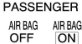
When the vehicle is started, the passenger airbag status indicator will light ON and OFF for several seconds as a system check.
