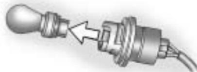
3. Pull the old bulb straight out of the bulb socket.
