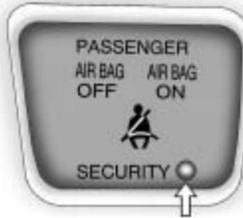
The security light is in the center of the instrument panel. It comes on if there is a problem with arming or disarming the theft-deterrent system.
