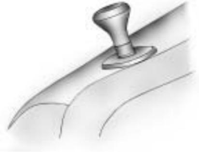
3. Pull up on the lock release knob, located on the top outboard side of the seatback.
