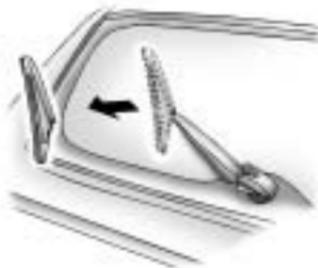
3. Push the rear wiper assembly straight into the rear wiper arm.
