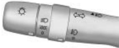
The lever on the left side of the steering column operates the exterior lamps.
