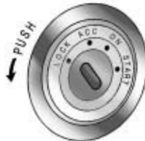
**Notice:** Using a tool to force the key to turn in the ignition could cause damage to the switch or break the key. Use the correct key, make sure it is all the way in, and turn it only with your hand. If the key cannot be turned by hand, see your dealer/retailer.
