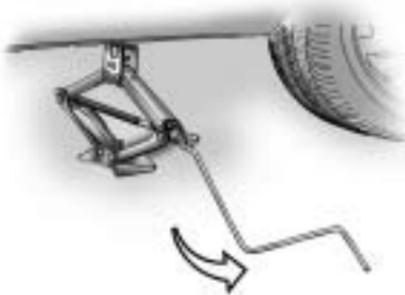
13. Turn the jack handle counterclockwise. Lower the jack completely.
