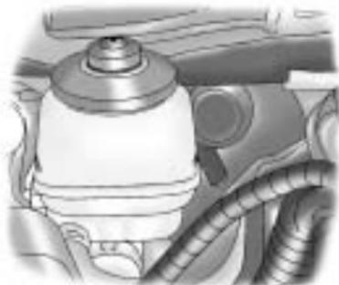
The reservoir is located at the back of the engine compartment, on the driver side of the vehicle. *Engine Compartment Overview on page 9-6.*
