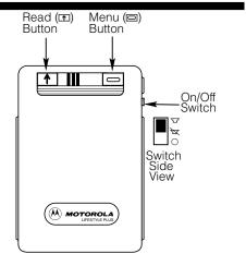
**READ Button:** (**ID**) - Used to read messages and to activate pager functions. Also used to scroll through the hours and minutes digits for time setting.
