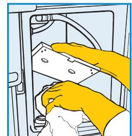
**10** • Clean interior of refrigeration unit. Remove and clean trays, and wipe down tubing with a sanitized\* towel. Reinstall trays.
