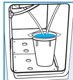
**9** • When the display changes to "INSERT FRESH WATER," remove the empty cup and replace it with the cup containing plain hot water. Press **CLEAN** button.
