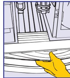
**9.** When the brew cycle is finished, open the front doors of machine, clean the drain tray and grate. Remove and empty the grounds bin, and replace it in the machine.
