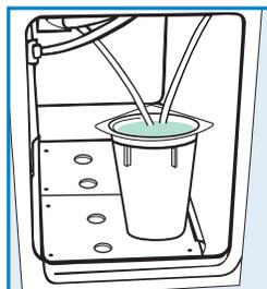
**7** • Place both milk tubes into the cup with Cleaner #1. Press **CLEAN** button.
