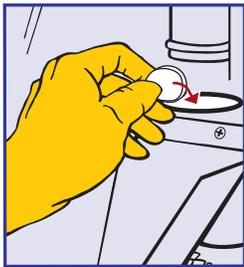
**6.** Place one Cleaning Tablet in the brew chamber. DO NOT mistakenly place the tablet in the grounds chute or coffee funnel.
