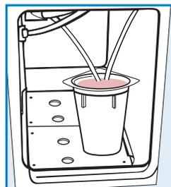
**8** • When display changes to "INSERT CLEANER #2," remove the first cup and replace it with the cup containing Cleaner #2. Press **CLEAN** button.
