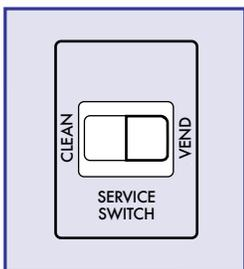
**11.** Press the service switch to the "VEND" position. Secure cleaning materials and close all doors. The brew system cleaning process is now complete.
