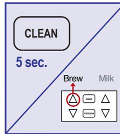
**4.** Press and HOLD **CLEAN** button for 5 seconds until tone stops. Select "BREW" by pressing left **▲** button.
