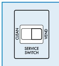
**13** • Press the service switch to the "VEND" position. Secure cleaning materials and close all doors. The milk system cleaning process is now complete.
