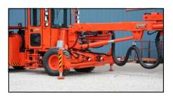
Sealed, pressurized, heated and air conditioned cabs with **HEPA filtration meet NIOSH** recommendations in their publication #2008-10. This provides a clean, quiet working environment increasing operator comfort and reducing operator fatigue.
