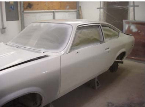
Wet coat of Supafil primer reduced out thinner to act as a sealer then sanded with 400 grit
