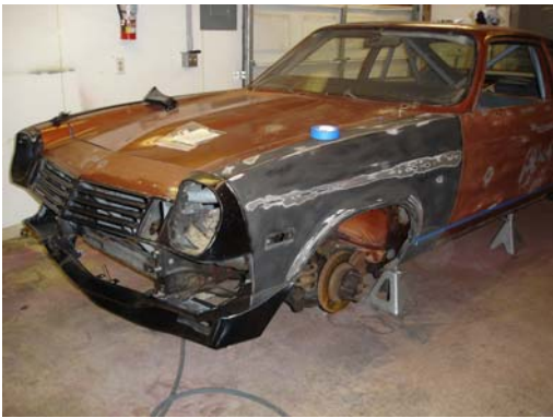
Replaced damaged front fenders, and sanded whole car with 220 grit on a DA sander
