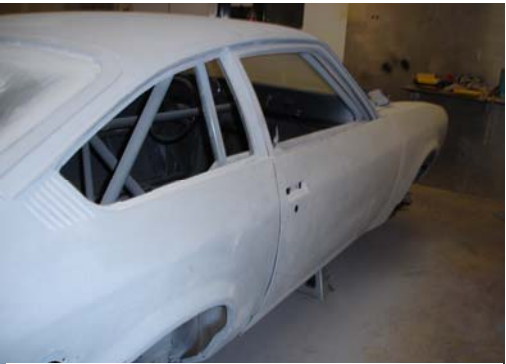
Heavy coats of Supafil primer and lots of sanding with 220 grit to get it (near) straight
