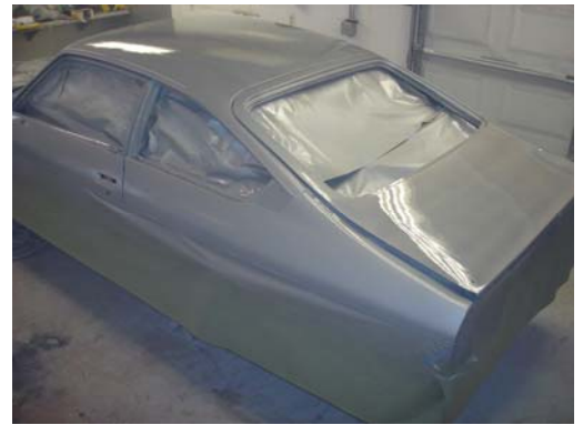
Masked off and top coat of Cosworth silver applied
