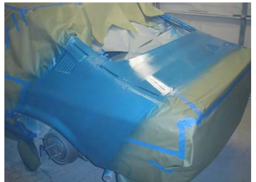
Masked off for the final color coat, Cosworth blue (continued on pg. 8)
