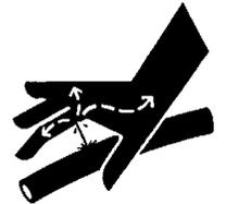
Do not search for hydraulic leaks without body and face protection. A tiny, almost invisible leak can penetrate the skin, requiring immediate medical attention.
