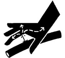
Do not search for hydraulic leaks without body and face protection. A tiny, almost invisible leak can penetrate the skin, thereby requiring immediate medical attention.
