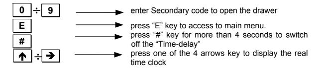
Generally is not requested to switch off using the drawer with "#" key: the device will switch off automatically after 60 sec. of non use.
