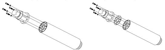
Figure 4.2 Removing the UMP
