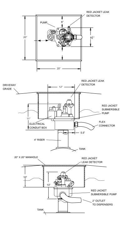
Figure 1.1 Leak detector and manifold dimensions
