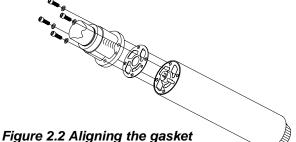
Figure 2.2 Aligning the gas
