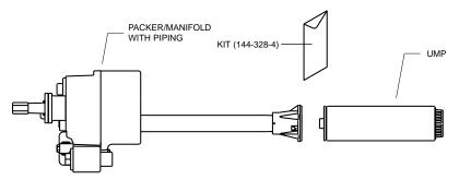
Figure 2.1 Attaching the UMP
