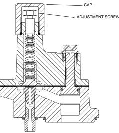
Figure 2.14 Functional Element cap and adjustment screw
