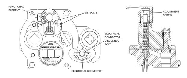
Figure 4.4 Packer with Functional Element
