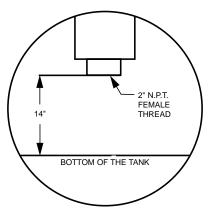
Figure 1.3 Floating Suction Adapter
