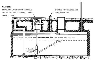
Figure 1.2 Floating suction installation
