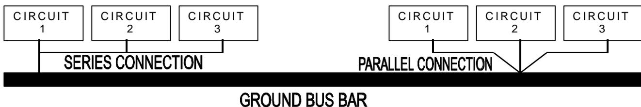
Figure 3-Single Point Ground Types
