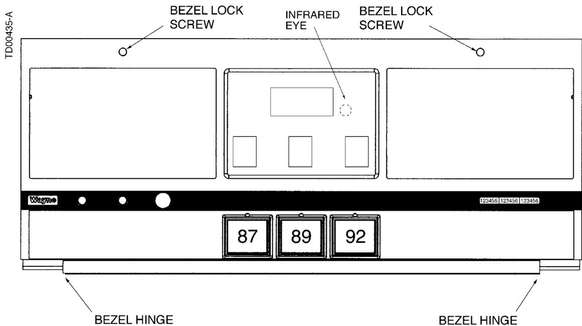
**FIGURE 6-2. INFRARED INTERFACE LOCATION.** The dispenser infrared eye is located behind the sales display on each side of the dispenser.
