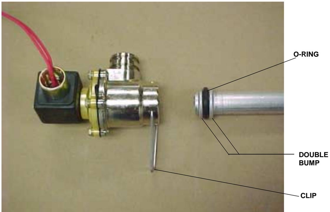
FIGURE 5-4. DOUBLE BUMP TUBE BETWEEN VALVE AND HOSE OUTLET.
