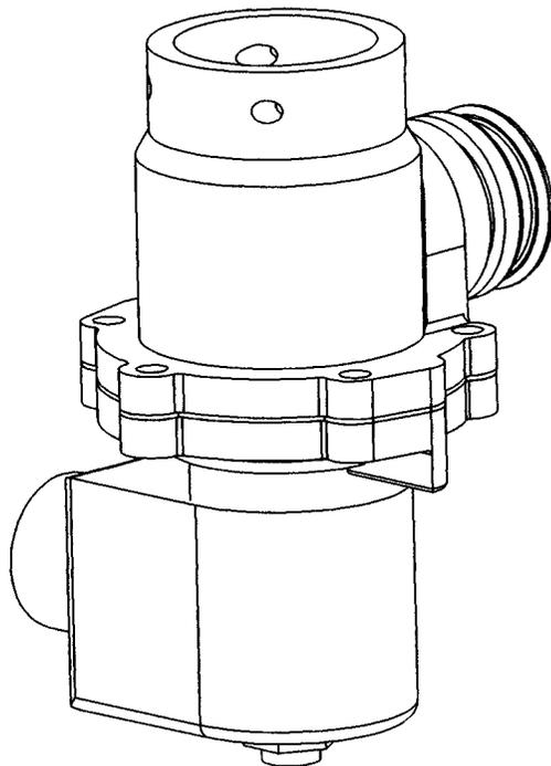
**FIGURE 5-2. PROPORTIONAL FLOW CONTROL VALVE.** *In 3/Vista models the valve is located at the meter outlet.*
