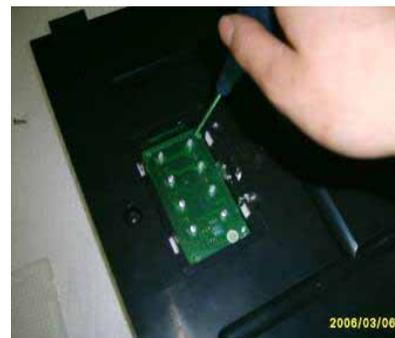
4. Loosen the screws which fixed on the display panel.
