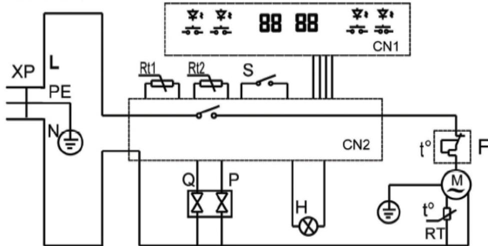
XP-Power Plug CN1-Display panel CN2-Control Panel S-Lamp switch
