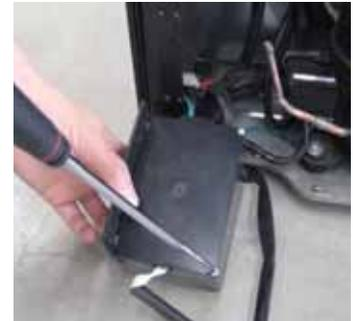
3. The main control panel is fixed in the panel box by a screw, dismantle it ,the control panel will be removed
