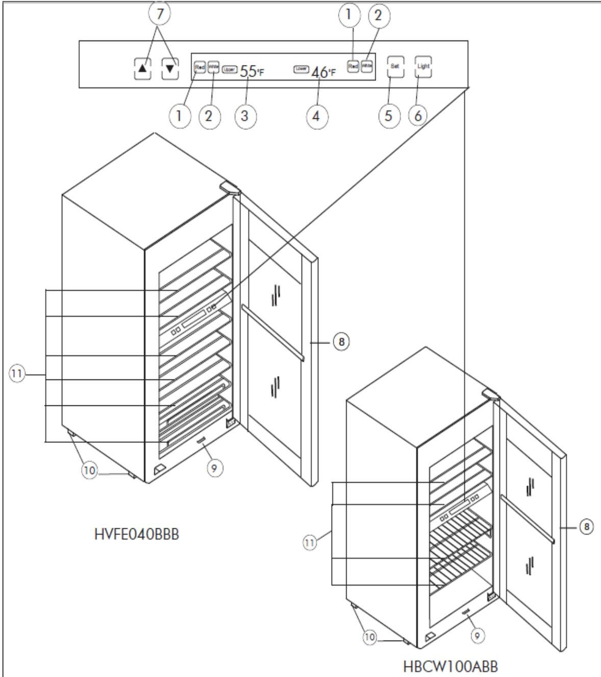
Once we plugged the unit, it needs to run for 30 minutes at least to acclimate itself before any adjustments. During this time, depending on the internal temperature, the red or white wine light will stay on for the upper compartment and red or white wine light will stay on for the lower. The LED display will show the current internal temperature.
