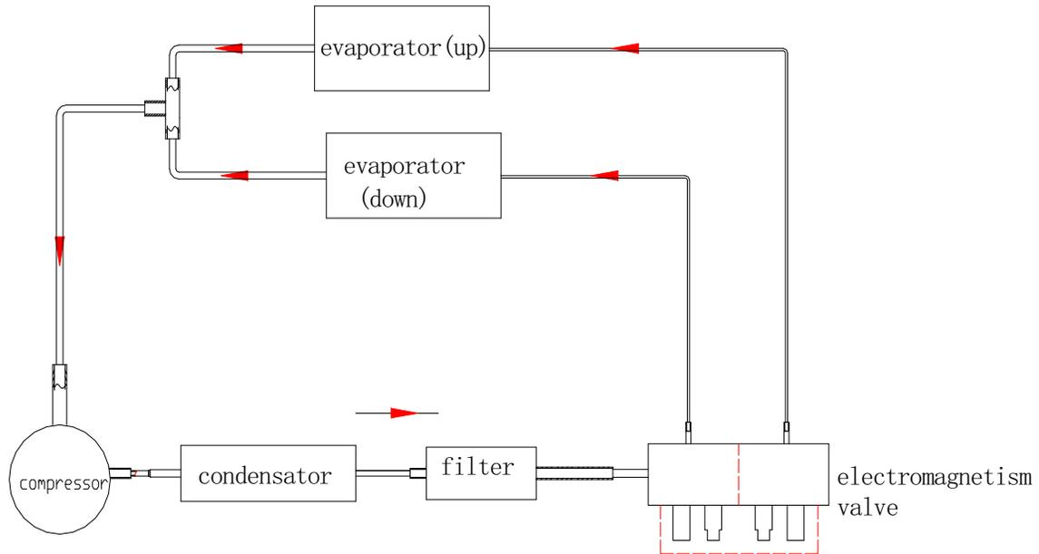
Explanation: The electromagnetism valve includes two single valves. When the two compartment temperature does not reach the set temperature, the two valves are keeping open; when one compartment temperature reaches the set temperature, the related valve is closed and the other one is keeping open. Both the two compartments temperature reaches each set temperature; the valves don't close but the compressor stop working.
