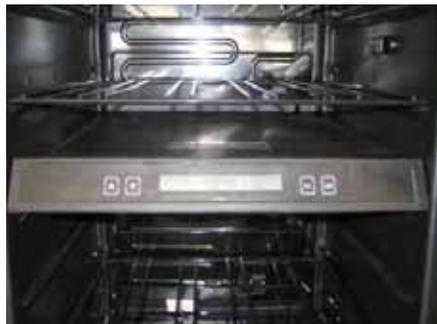
1. The middle partition is fixed on the cabinet with two screws, so you should loosen the screws and take off the middle partition from the unit.
