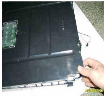
3. Disassemble the lampshade from the low lid, and loosen the screws fixed the LED light.
