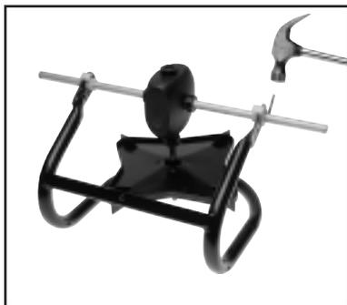
**5.** Install the wheels. Be sure slotted hub side is next to the frame. (The drive pin will engage the drive wheel.)
