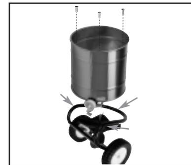
**8.** Install front center bolt & nuts (2-4) along with the front grab handle (52) (loosely) first. Then install side bolts, and tighten all bolts securely.
