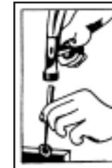
To re-use hubcap, place round punch in lock tab opening. Strike lightly. Deform each tab 1/32".
