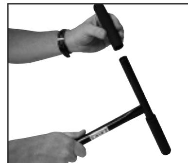
**10.** Connect T-handle to center section using (1) 1 1/4" bolt and nut.
