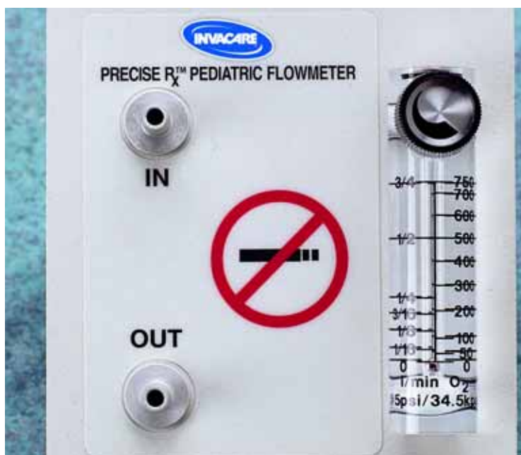
Detail of Invacare PreciseRx pediatric flowmeter
