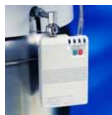
The Venture DODD can also be used on liquid-oxygen reservoirs.
