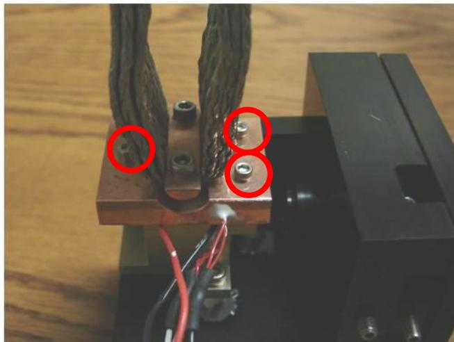
*Figure 24: Three fasteners secure TMA to YAG crystal holder*
