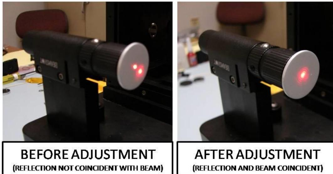
*Figure 30: Beam and Reflection Coincidence*
