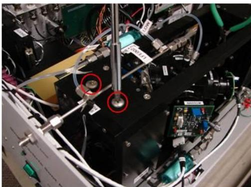
*Figure 8: Coupler Chamber Sealing Screws*
