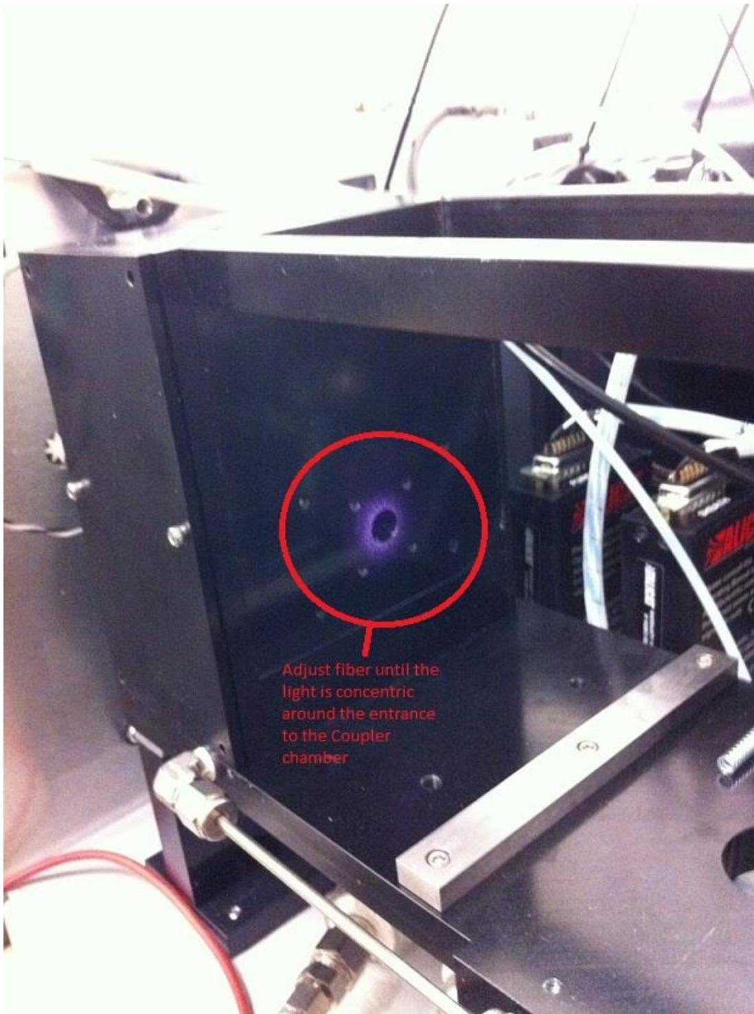
Figure 32: Light Concentric Around Entrance to Coupler Chamber
