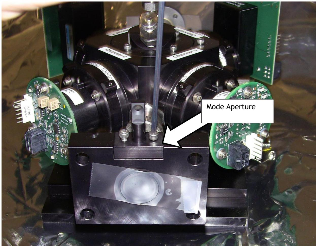
Figure 5: Installing Mode Aperture in Upside-Down Position
