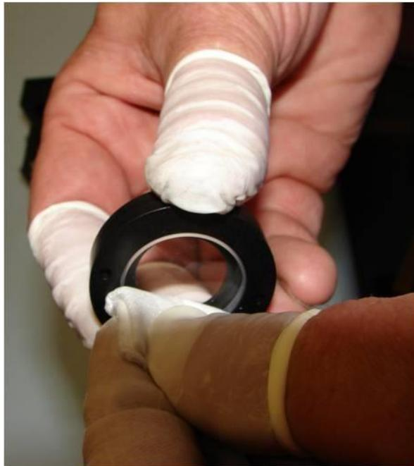
*Figure 21: Wiping the output coupler*
