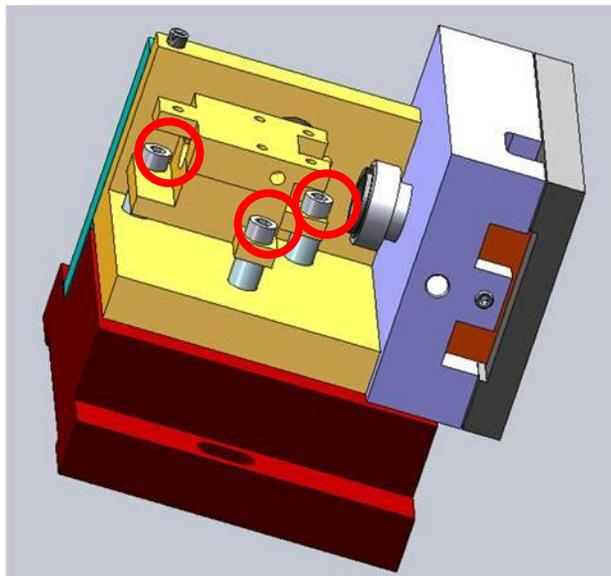
Figure 23: Fasteners securing YAG crystal holder to pump base
