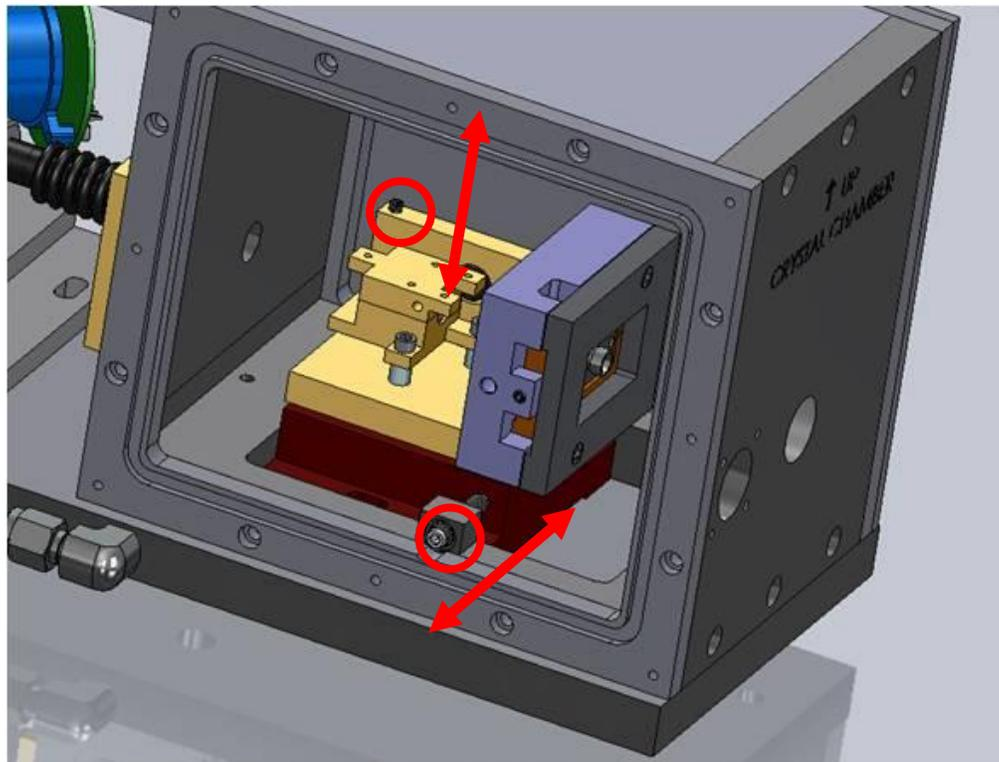
Figure 29: Adjusters that aim the YAG Crystal Assembly (thermal management assembly removed for clarity)
