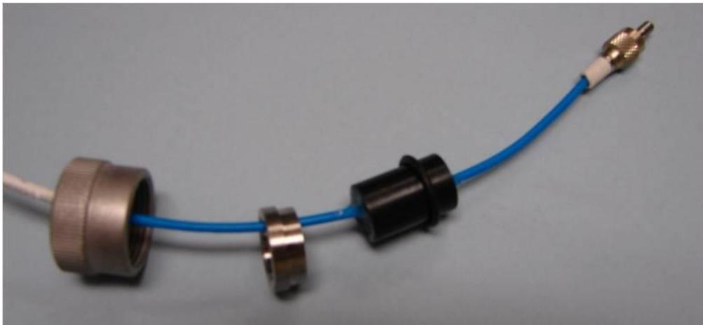
*Figure 17: Components of Fiber Passthrough*
