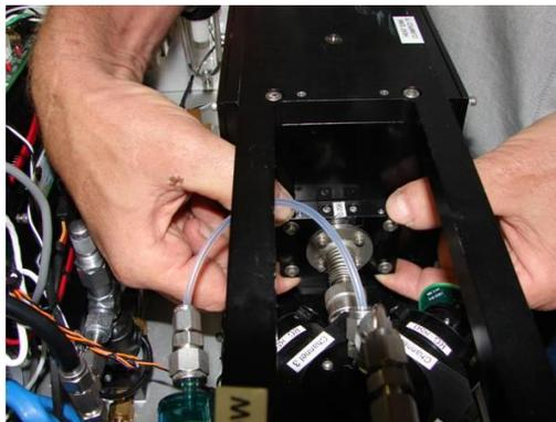
Figure 12: Manual mode aperture alignment
