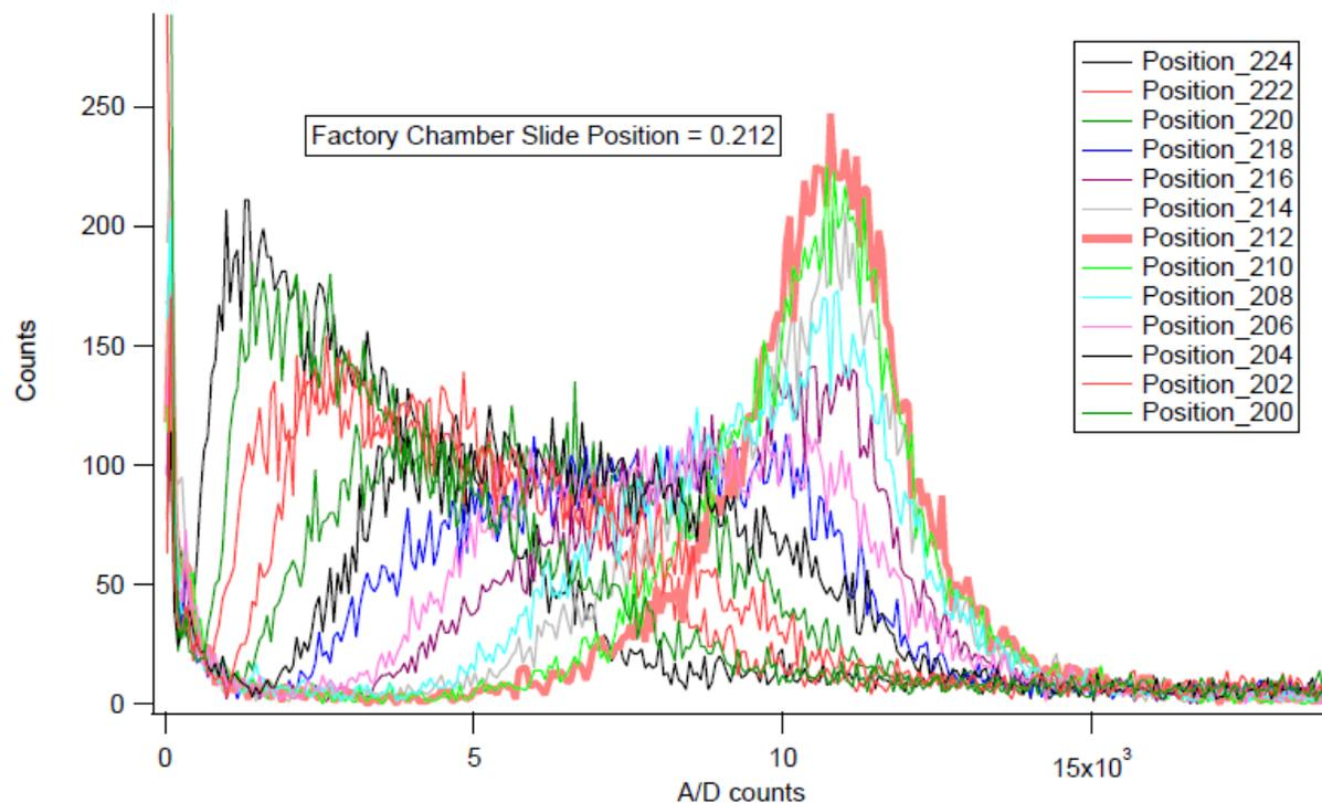
Figure 14: Histogram Response as Chamber Plate is Translated
