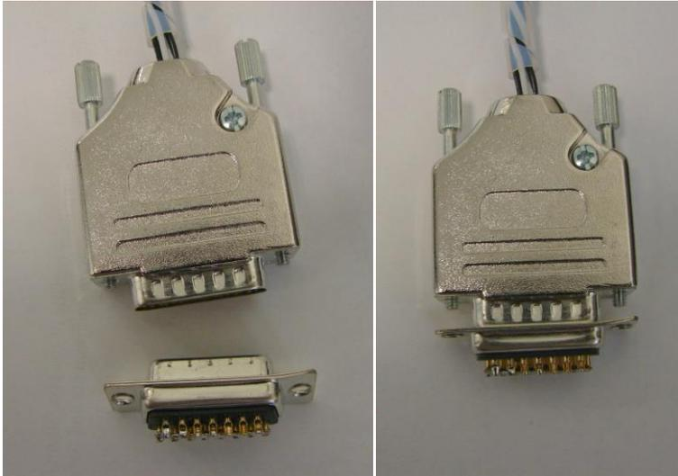
*Figure 36: Shorting Plug Detached (left) and Attached (right) to Power Connector*
