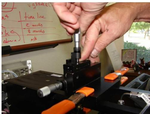
Figure 13: Application of extra force to assist stage springs
