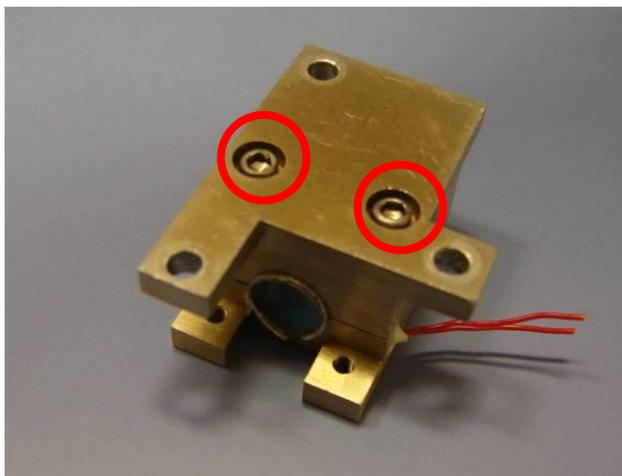
*Figure 25: Screws securing halves of YAG Crystal Holder together*
