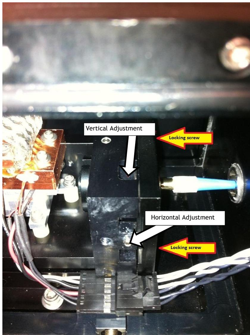
Figure 33: Locking and Adjustment Screws
