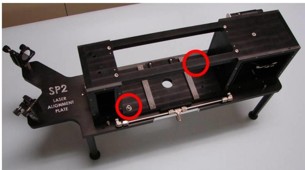
Figure 19: Frame-to-fixture fasteners
