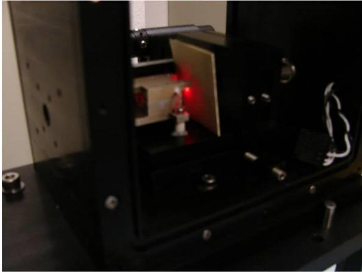
Figure 28: Paper between Crystal and Mode Match Optics
