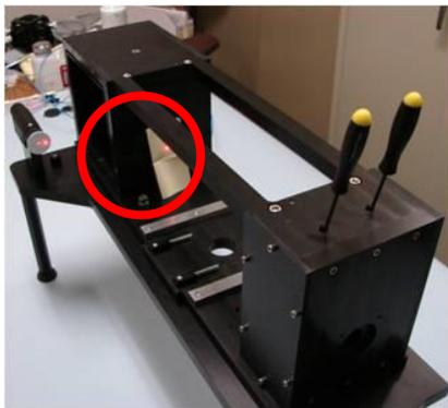
Figure 31: Paper Placed to Block Reflection from Crystal Face
