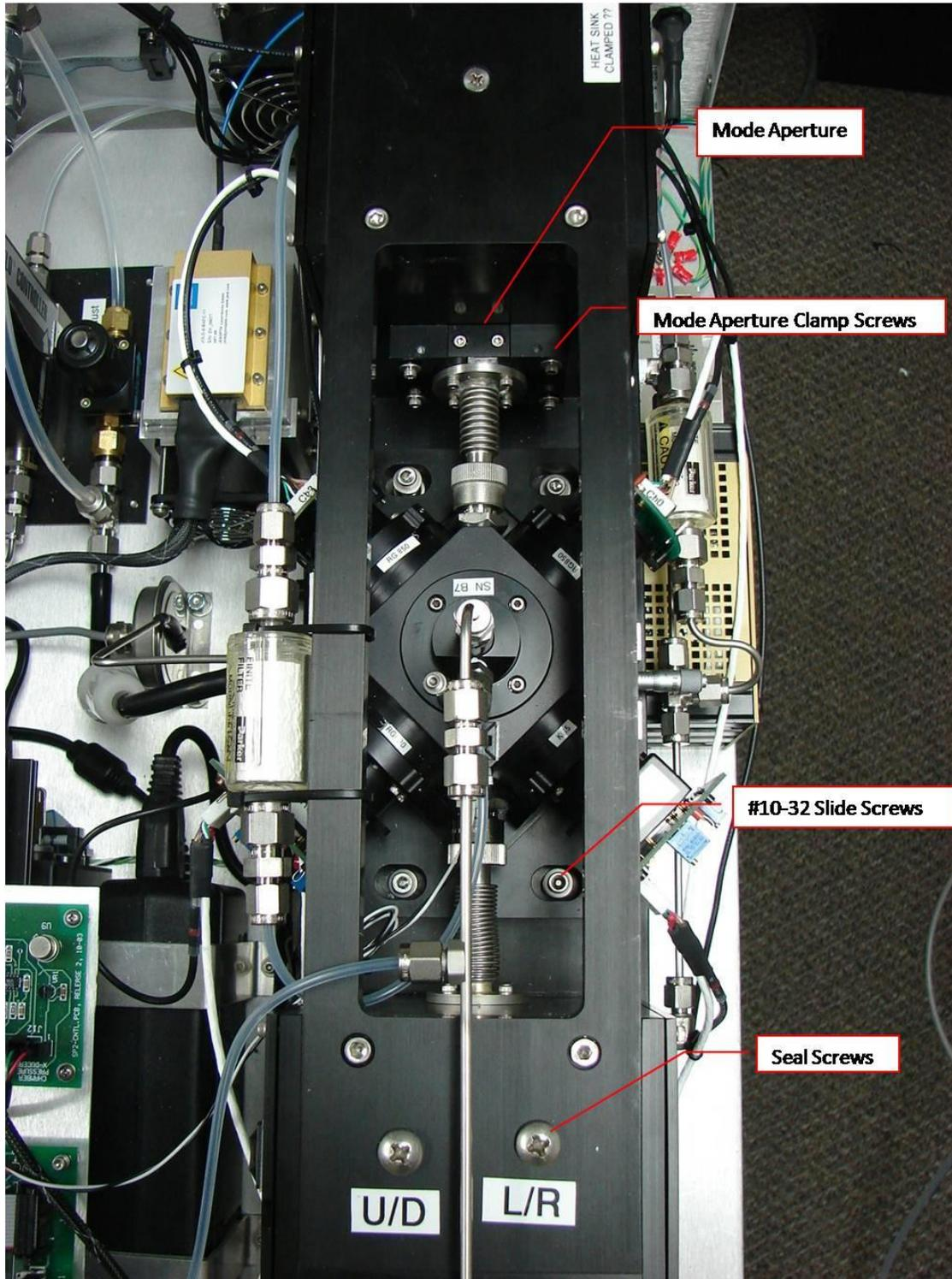
Figure 3: SP2 Spectrometer Head
