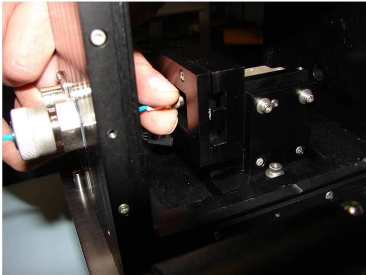
*Figure 16: Unscrewing SMA Connector*
