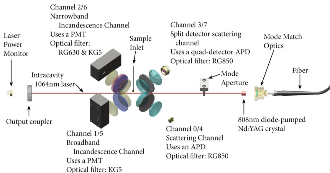
Figure 1: Nd: YAG Laser Resonator Cavity
