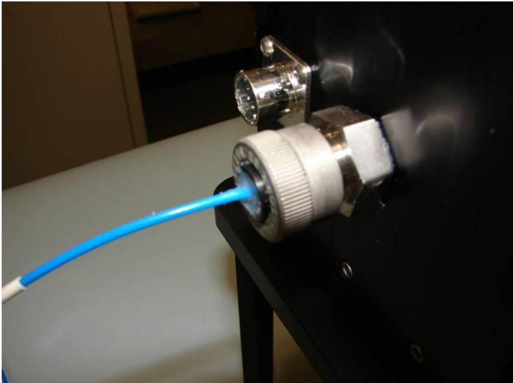
*Figure 15: Ultra-Torr Fiber Passthrough Fitting*
