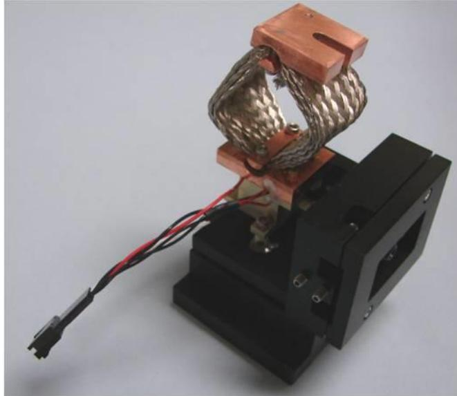
*Figure 22: YAG Crystal and Optical Pump Assembly*
