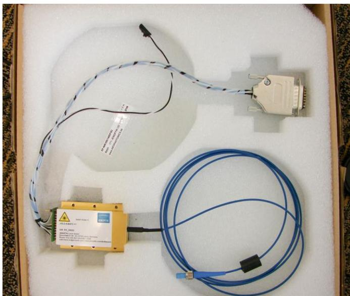
Figure 35: SP2 Pump Laser in Protective Box
