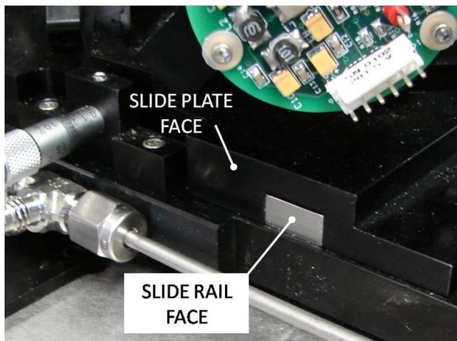
Figure 34: Centered chamber (coplanar slide plate and slide rail end faces)
