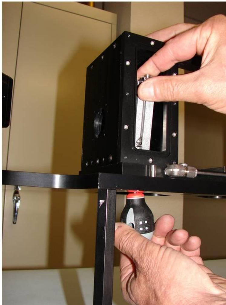
Figure 20: Removing Output Coupler Mounting Screws
