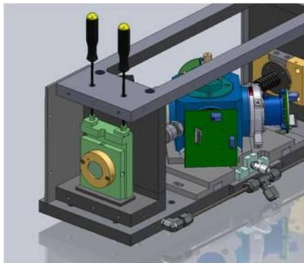
Figure 9: Tip/tilt adjustment of output coupler mount
