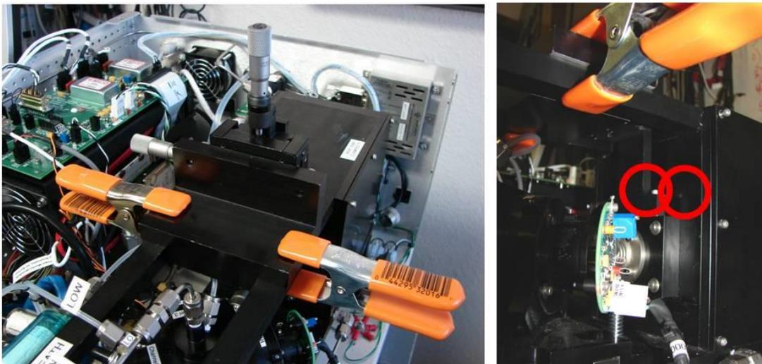
Figure 11: Attachment of Mode Aperture Alignment Tool
