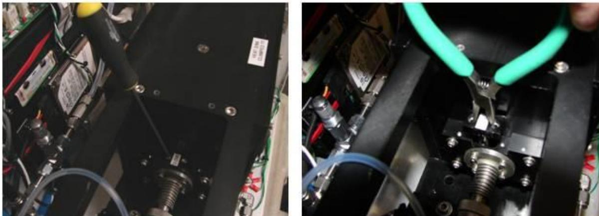
*Figure 4: Mode Aperture Removal*
