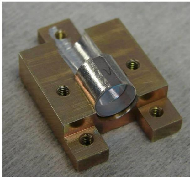
Figure 26: YAG Crystal cushioned in holder
