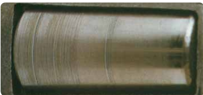
Circular wear on the roller, the result of hard particle contamination in the lube.
