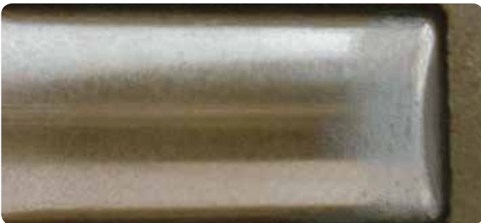
Small end of the roller shows excessive wear, the result of loose bearing adjustment.
