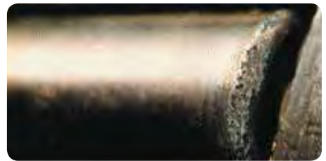
Roller end cracks indicate excessive loading or excessive misalignment.
