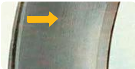
Severe sliding wear due to presence of hard abrasives.
