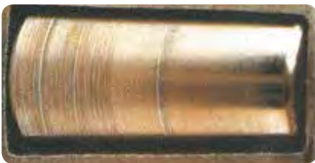
Scoring indicates contamination by dirt, grit or metallic particles.
