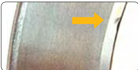
Dings and dents in the bearing surfaces indicates a drift was used during installation.
