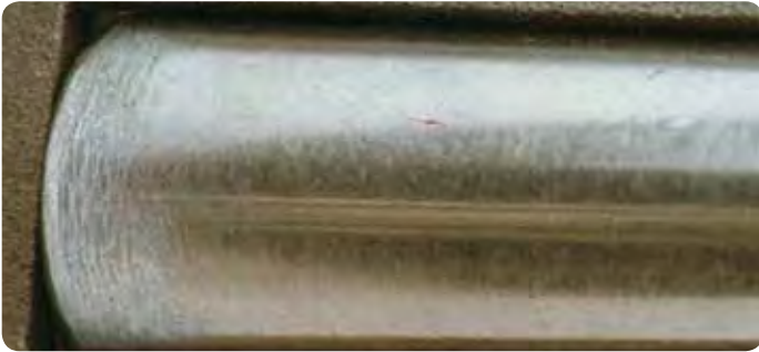
Large end of roller shows scoring, the result of excessive preload.
