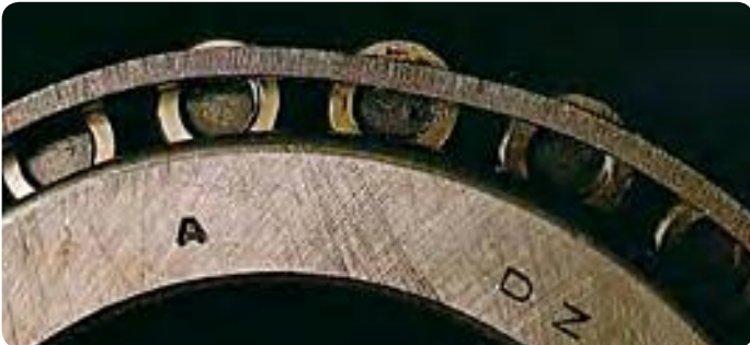
Deformation of the cage, the result of improper installation or mishandling prior to installation.
