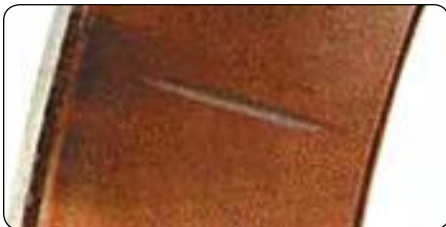
Dent across the race indicates a sharp high impact.
