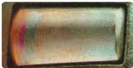
Coloration indicates an overheated bearing - from straw brown to deep purple. Causes are lack of lubricant, misadjustment or excessive loading.
