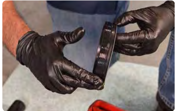
Lightly lubricate the OD and ID with the fluid being retained.
