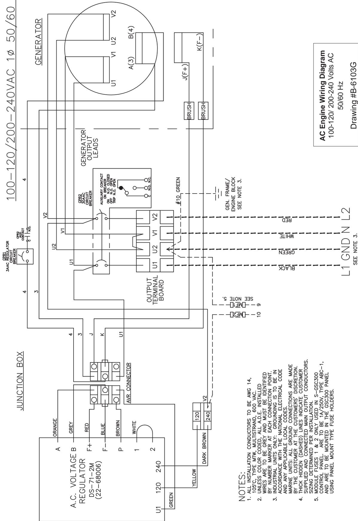
**AC Engine Wiring Diagram**
