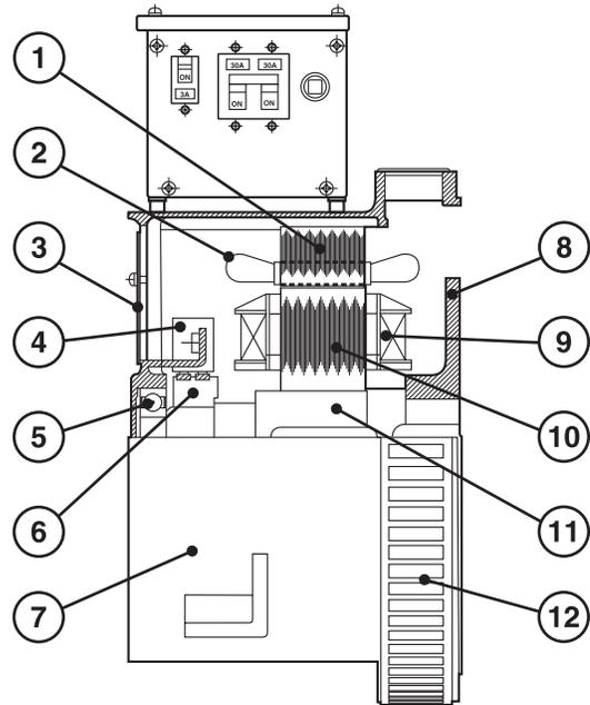
Figure 24: Generator Components.
