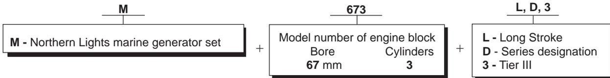
**M673L3** = Northern Lights marine diesel generator set with a 673 engine long stroke, TF-276D generator end, Tier III.
