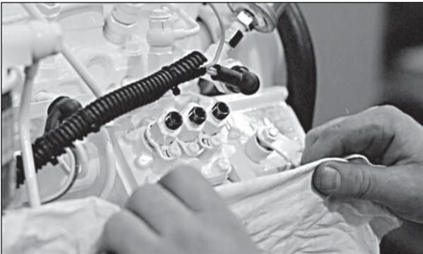
**Figure 15:** Cover lines, inlets and injection pump outlets.
