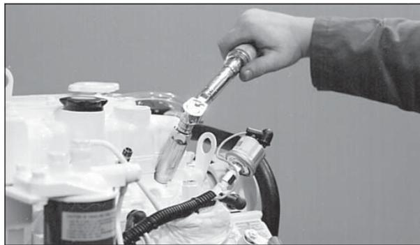
**Figure 20:** Reinstall injector. Torque to proper tightness.
