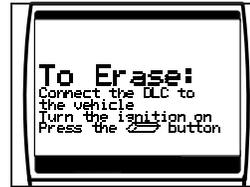
1. If not connected already, connect the Scan Tool to the vehicle's DLC, and turn the ignition "On." (If the Scan Tool is already connected and linked to the vehicle's computer, proceed directly to step 4. If not, continue to step 2.)
