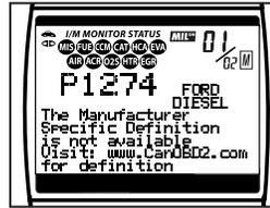
10. If more than one DTC was retrieved, and to view Freeze Frame Data, press and release the **DTC SCROLL**
